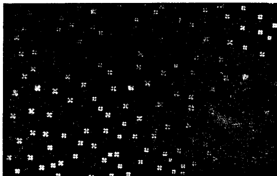
Figure 4. The smectic A phase appearing from the isotropic phase in the form of tiny spherical droplets in a mixture of 80CB and DODA in the molar ratio of 50:50. Crossed polarizers ( \times 150 ).
