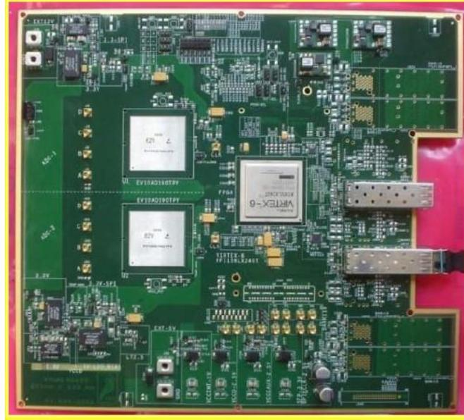
Fig. 3. Photograph of the pSPEC board.
