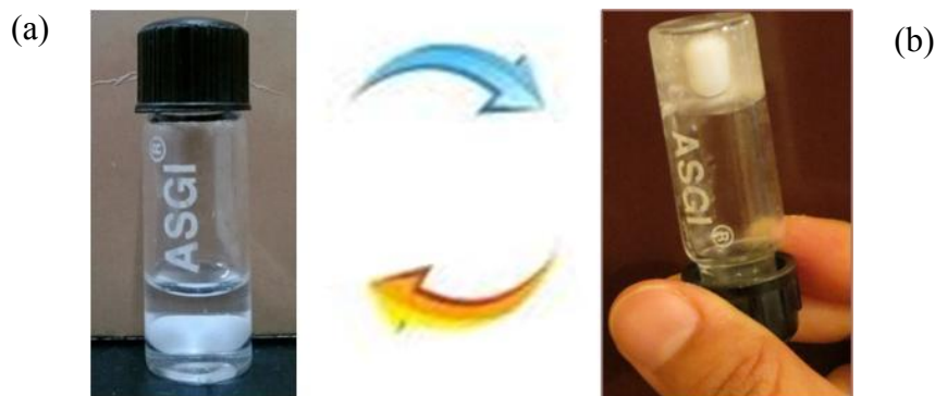
Figure 1. Photographs of the vial containing the colloidal suspension and a teflon coated magnetic pellet at (a) T > 60^\circ\text{C} and (b) RT
