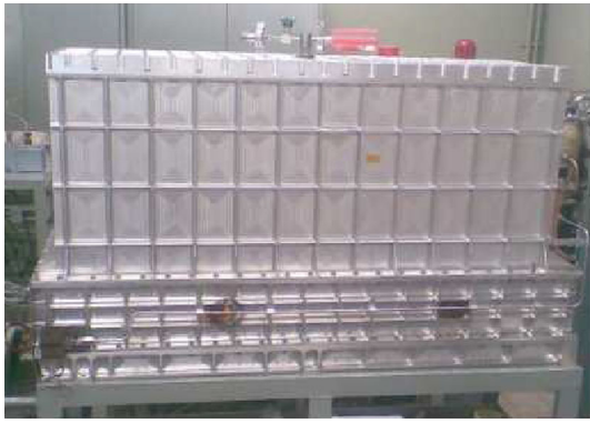
Figure 4. Photograph of a fully assembled LAXPC detector without tin shield.
