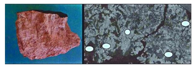
(Left) A fragement of the Piplia meteorite. The black surface on the top is crust produced by theheating and burning that occurs during its atmospheric transit. (Right) A slice of the meteorite showing the portions where material was taken out for analysis.
