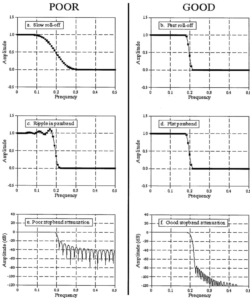
Parameters for evaluating frequency domain performance. The frequency responses shown are for low-pass filters. Three parameters are important: (1) roll-off sharpness, shown in (a) and (b), (2) passband ripple, shown in (c) and (d), and (3) stopband attenuation, shown in (e) and (f).
