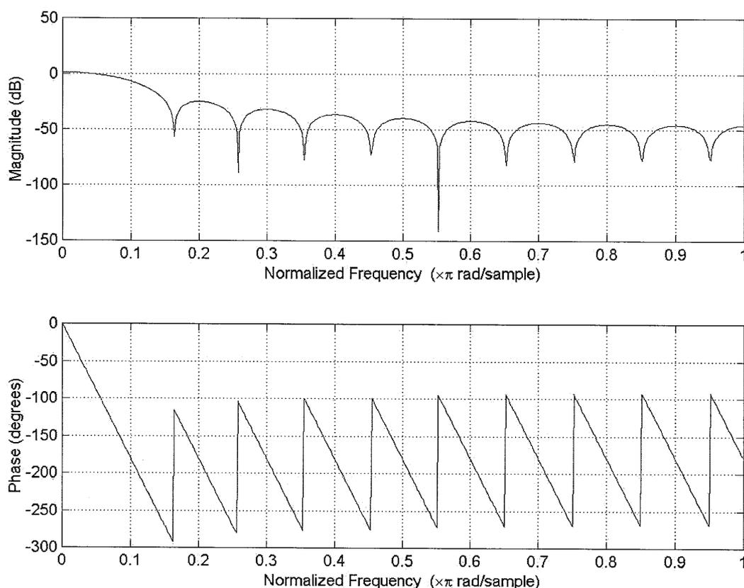
From the above plot we find that the filter response in the pass-band is not flat, which implies that the number of taps  $N$  must be increased. The taps were increased in the filter and it was found that at  $N=113$  the filter response was flat in the pass-band. The response for the filter with taps  $N=113$  is as given below
