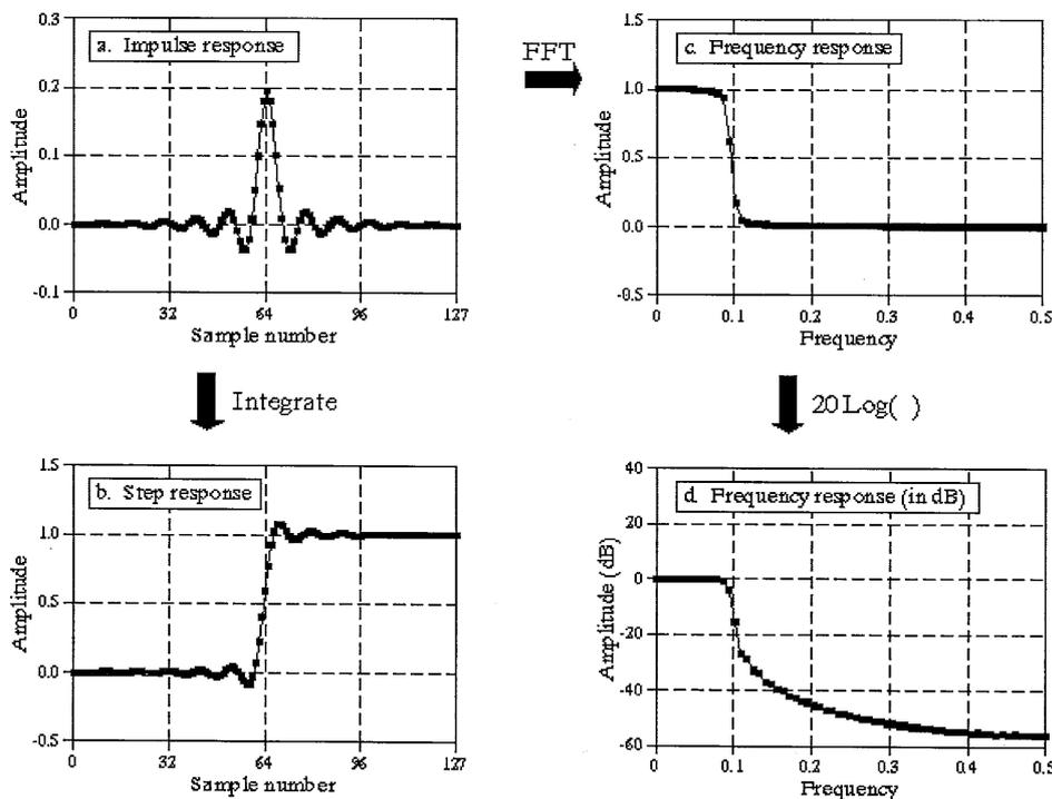
Filter parameter (a). Impulse response, (b). Step response, (c) The frequency response of the (c). impulse response (d). step response in dB.
