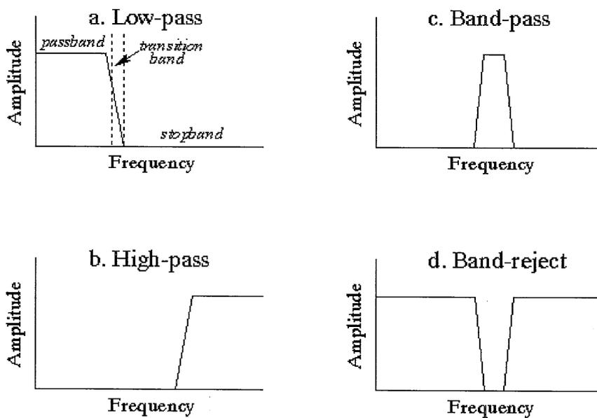
Figure shows the four basic filters response **a.**low-pass, **b.**high-pass, **c.**band-pass, and **d.**band-reject.
