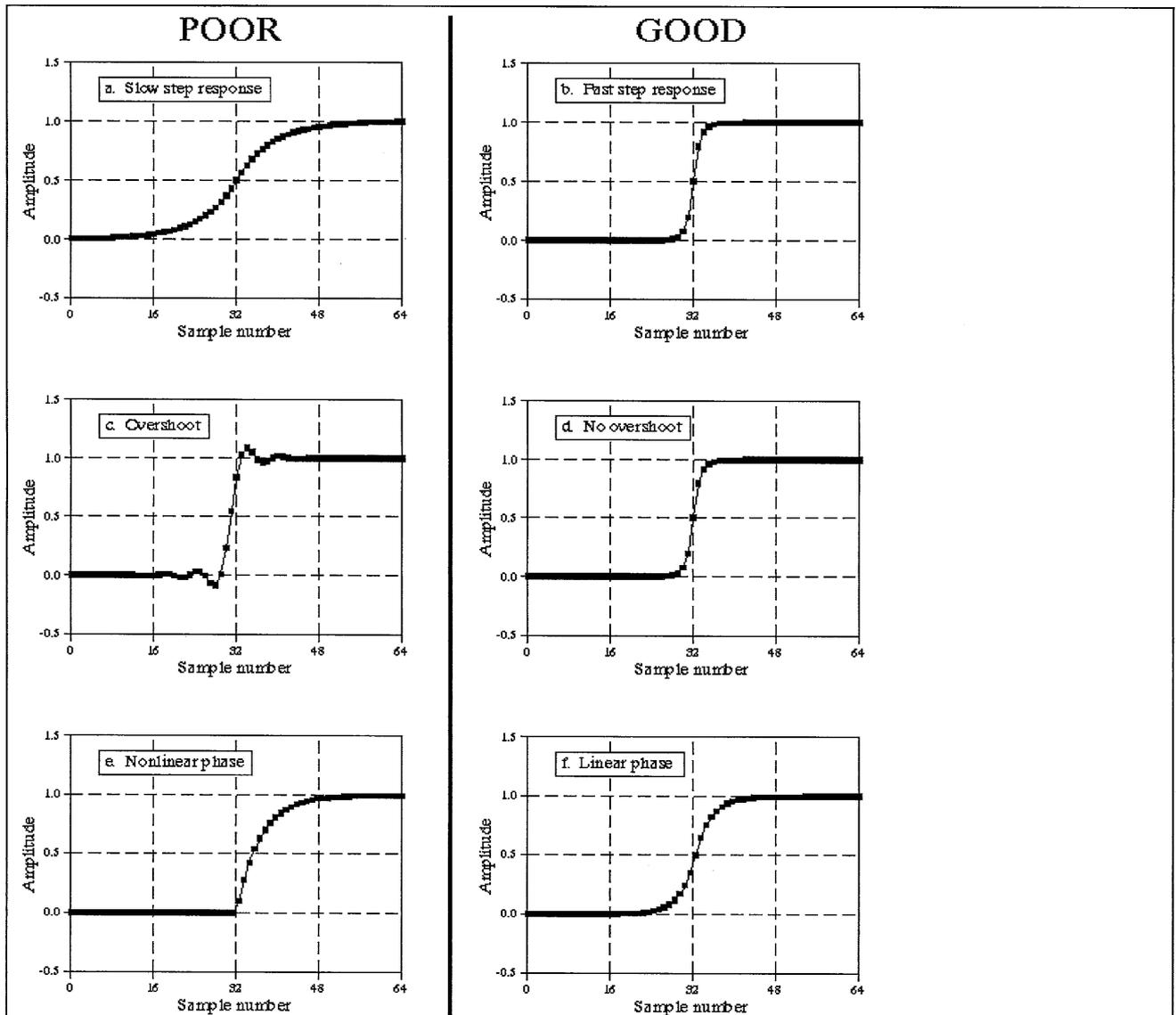
Parameters for evaluating time domain performance. The step response is used to measure how well a filter performs in the time domain. Three parameters are important: (1) transition speed (risetime), shown in (a) and (b), (2) overshoot, shown in (c) and (d), and (3) phase linearity (symmetry between the top and bottom halves of the step), shown in (e) and (f).
