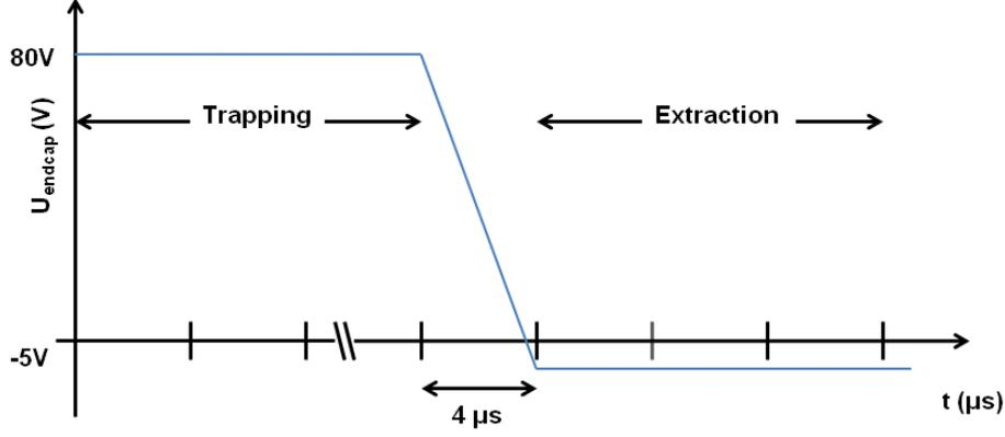
**Figure 4.4:** Endcap voltage transient time is about  $4\mu\text{s}$  and is assumed to be linear.
