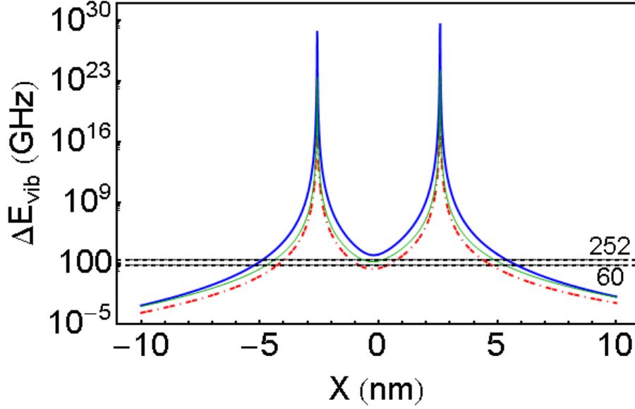
**Figure 6.5:** In (b) we see the variation of the vibrational energy transferred to the molecule as a function of  $X$ , plotted for ion velocities of 1, 500 and 1360 m/s in blue, green and dashed red lines.
