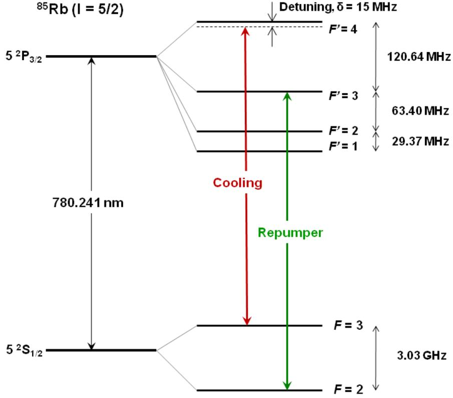
**Figure 3.4: Rb D2 line manifold:** illustrates hyperfine structure, with frequency splittings between the hyperfine energy levels (not in scale) [45].
