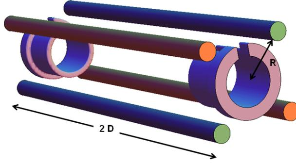
**Figure 3.16:** The SIMION 7 rendering of the ion trap geometry is shown. Four long parallel rods are arranged in a quadrupole configuration. Endcap ring electrodes are along the axial direction.
