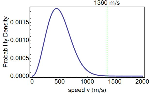
**Figure 5.7:** Maxwell-Boltzmann speed distribution of temperature  $\approx 1000\text{K}$  is plotted. The maximum trappable speed corresponding to  $0.8\text{ eV}$  matches the tail of the distribution of trapped ions.
