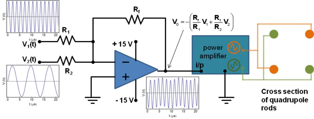
**Figure 3.23: Experimental setup to add a weak excitation frequency:** An Op-Amp adder circuit is used for adding two signals: RF drive voltage,  $V_1$  and a weak excitation frequency signal,  $V_2$ .  $R_1 = R_f = 4.7 \text{ k}\Omega$  and  $R_2 = 47 \text{ k}\Omega$ . Output signal of the adder,  $V_0 = - (V_1 + \frac{1}{10} V_2)$  is fed to the power amplifier, which splits the signal into two signals with opposite phase.
