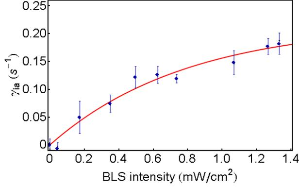
**Figure 5.4:** (color online) A subtraction of the data in Fig. 5.2 from that in Fig. 5.3 is plotted to isolate the ion-atom interaction term. This loss rate coefficient of the MOT atoms due to ion atom interaction,  $\gamma_{ia}$  is plotted against BLS intensity,  $I_{pi}$ .  $\gamma_{ia}$  is fitted with a single exponential function of the form, Eq. (5.21) and the coefficients of the fit are utilized to characterize the interaction term, as discussed in the text.
