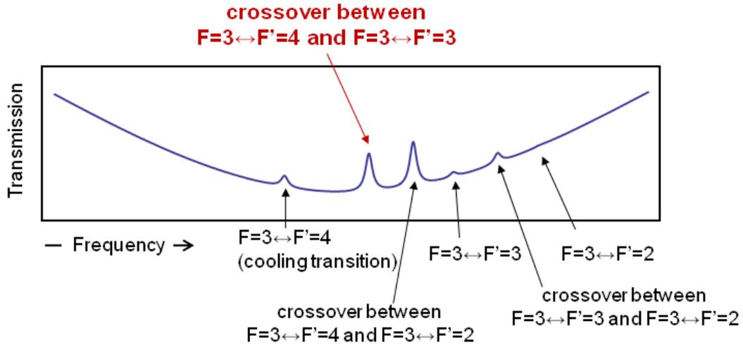
**Figure 3.5: Saturation absorption spectroscopy spectrum of  $^{85}\text{Rb}$ :** The spectrum shows transition lines between  $|5^2S_{1/2}, F = 3\rangle \rightarrow |5^2P_{3/2}, F'\rangle$ . The experimental setup of saturation absorption spectroscopy is shown in Fig. 3.6. The laser frequency is locked to the crossover between  $F = 3 \leftrightarrow F' = 4$  and  $F = 3 \leftrightarrow F' = 3$ .
