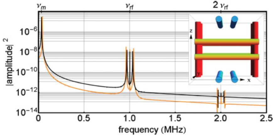
**Figure 2.5:** Power spectrum of the  $\hat{x}$  component of the trajectory for a low  $|\mathbf{v}_0|$  ion computed at  $\nu_{rf} = 1$  MHz,  $V_{rf} = 3$  V: (i) for the electrode configuration in Fig. 2.1 (a), black curve, and (ii) for the split electrode configuration in the inset, orange trace. For both power spectra, a strong macromotion peak at  $\nu_m$  and significantly weak peaks at  $\nu_{rf}$ ,  $\nu_{rf} \pm \nu_m$ ,  $2\nu_{rf}$  and  $2\nu_{rf} \pm \nu_m$  are seen.
