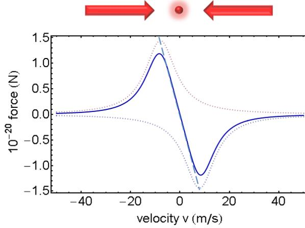
**Figure 3.1: Velocity-dependent force for an one-dimensional optical molasses:** Figure illustrates the scattering force as a function of velocity (solid lines) for a  $^{85}\text{Rb}$  atom in optical molasses where  $I = 3.5 \text{ mW/cm}^2$  per beam,  $\delta = 15 \text{ MHz}$  (below the resonance). The forces produced by each counter propagating laser beams are plotted as dotted lines.
