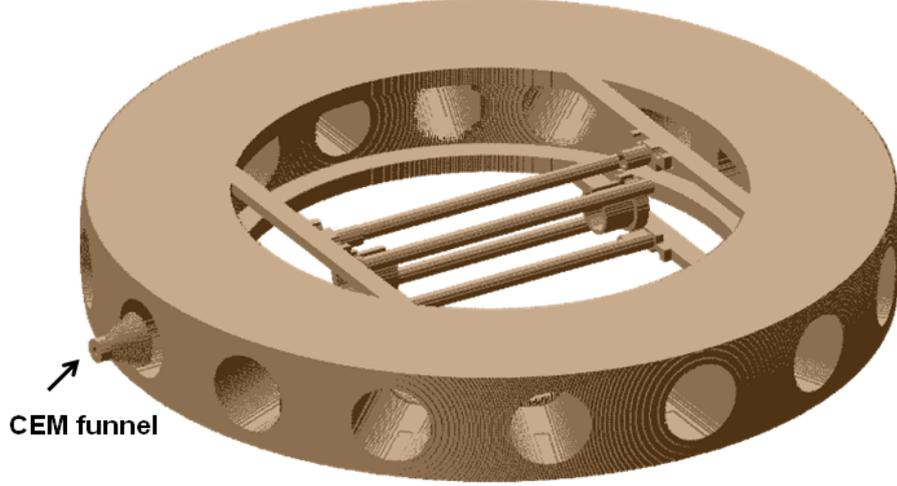
**Figure 4.2:** The SIMION 7.0 rendering of the ion trap geometry is illustrated.
