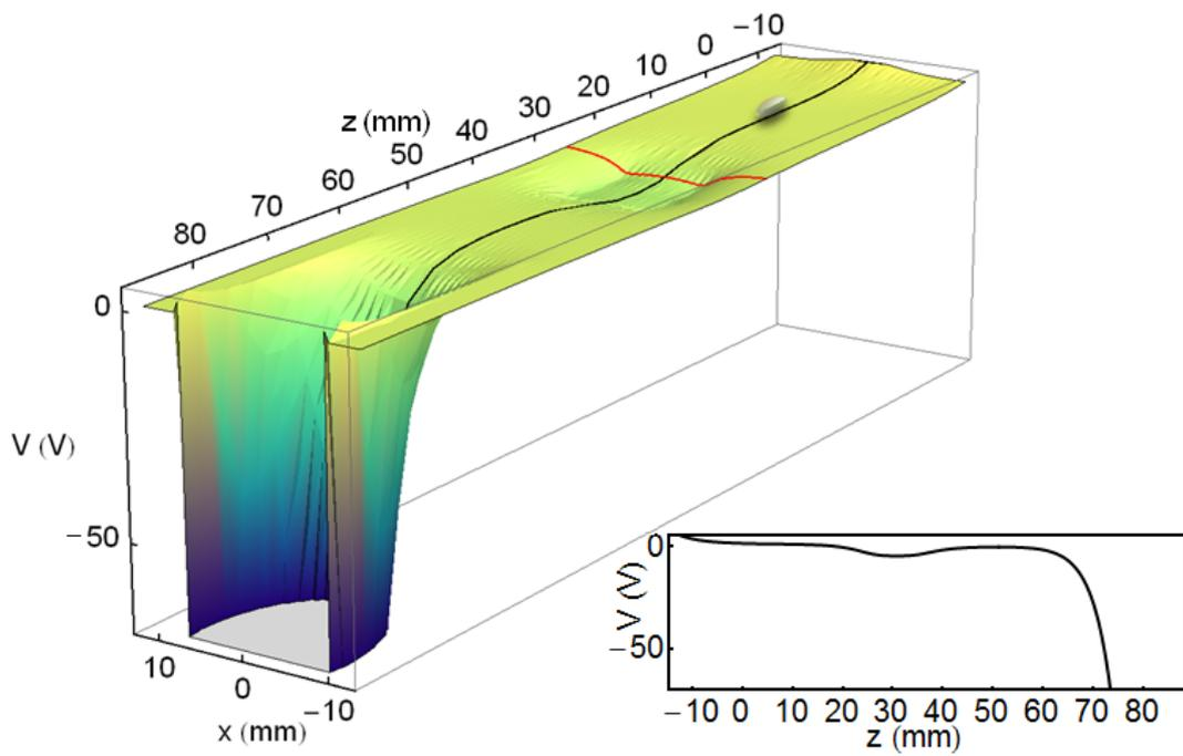
**Figure 3.22: Electric potential along z direction:** This potential is calculated for the CEM held at  $V_{CEM} = -2400$  V, one of the endcap electrodes near to the CEM at -5 V and opposite one at 80 V. A red line indicates the position of the extracting endcap electrode at -5 V. Ion cloud (not in scale) is drawn at the trap potential centre. The CEM is placed (not in the picture) at  $z = 87$  mm. A black line shows the potential along z direction, which is separately plotted in the inset.
