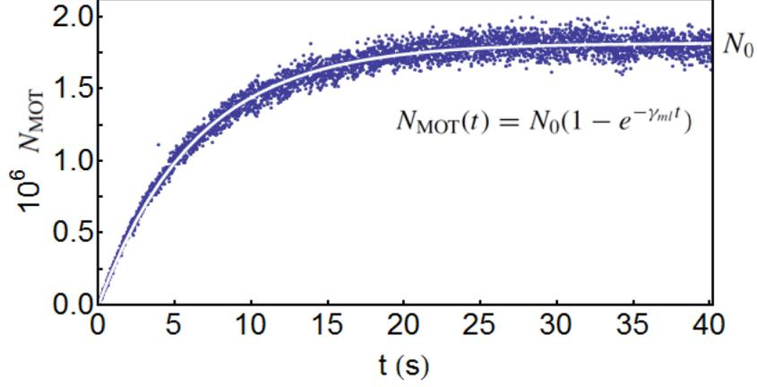
**Figure 3.10: Loading of atoms in the MOT:** Number of atoms in the MOT is measured by a photo-multiplier tube using spatial filtering technique, discussed in detail in Section 3.1.4.  $N_0$  is measured to be  $1.738 \times 10^6$  atoms, from which we derive  $L = 2.732 \times 10^5$  atoms/s and  $\gamma_{ml} = 0.157 \text{ s}^{-1}$
