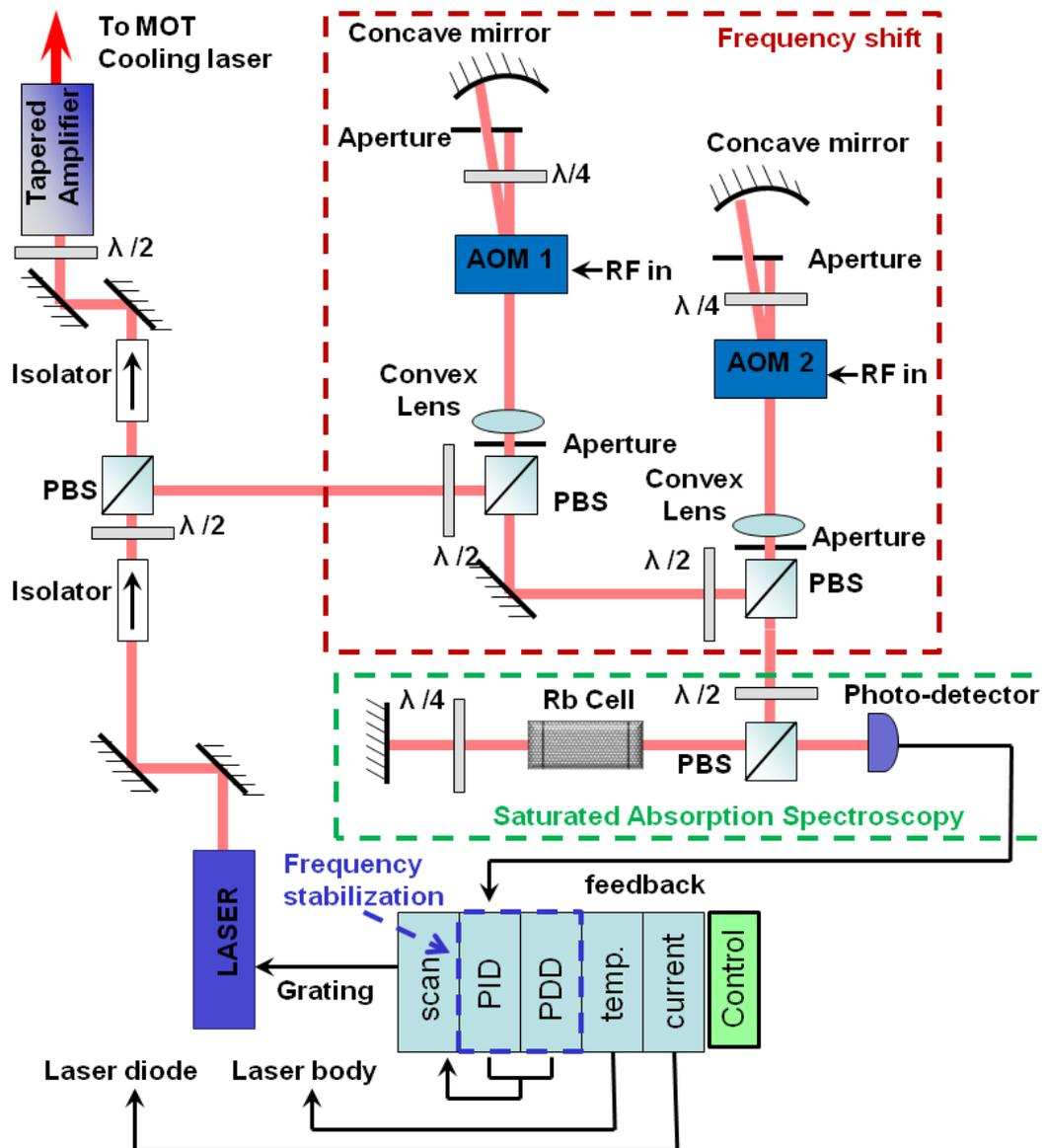
**Figure 3.6:** Schematic illustrates a set up to prepare the cooling laser with 15 MHz red-detuning to  $^{85}\text{Rb}$  D2 transition. The corresponding frequency shift of laser light is made using an acousto-optic modulator (AMO). Then this laser light is intensity-amplified by a tapered amplifier (TA) and sent to a MOT set up. Saturation absorption spectroscopy set up is shown in the green dashed box.
