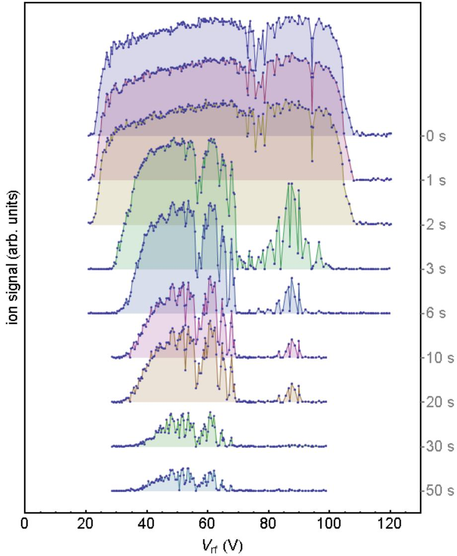
**Figure 3.27:** The experimentally determined stability region of the ions for 400 kHz scanned  $V_{rf}$  from 0 to 120 V for various holding times. The vertical axis is a measure of the number of ions detected after a 0.5s loading and immediate extraction.
