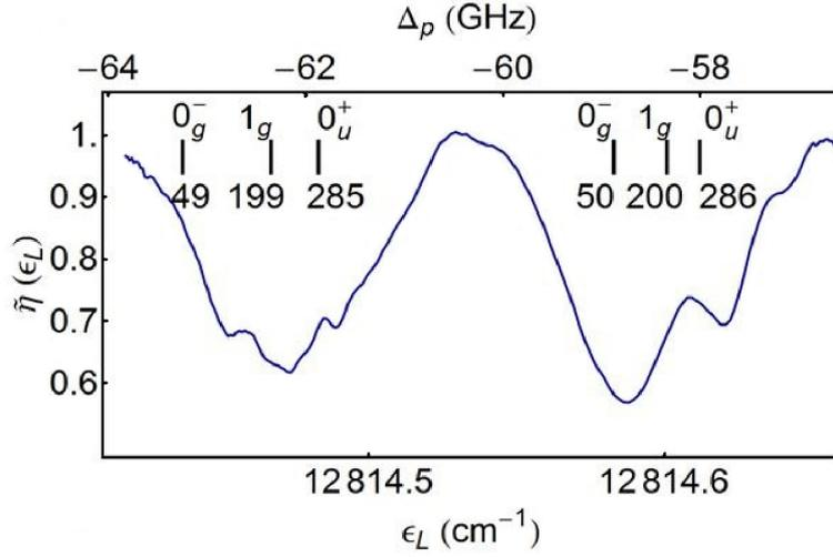
**Figure 3.31:** The change in MOT fluorescence  $\tilde{\eta}(\epsilon_L)$  is shown as a function of the photon energy of the PA laser  $\epsilon_L$ , scanned over these energies. The molecular states accessed in the present experiment are marked. When  $\tilde{\eta}(\epsilon_L) \approx 1$ , there is no molecule production. Dips in fluorescence correspond to the excitation of the molecular resonances.
