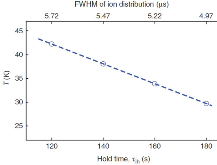
**Figure 4.12:** The trapped ion ensemble temperature is determined for the duration when the ion number has stabilized, that is for  $2 \leq \tau_{ih} \leq 3$  min. For this duration the temperature fit to the trapped ions as obtained from MD simulations (dashed line) is plotted as a function of trap hold time. The corresponding experimental ToF width of the extracted ions is marked on the top axis. The open circles represent the hold times at which the experimental measurements were made.
