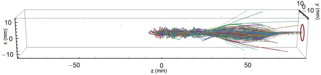
**Figure 4.8:** Ions are extracted toward the CEM through the endcap ring held at  $-5 \text{ V}$  and placed at  $z=51 \text{ mm}$ . A red ring in  $x$ - $y$  plane is a mouth of the CEM.
