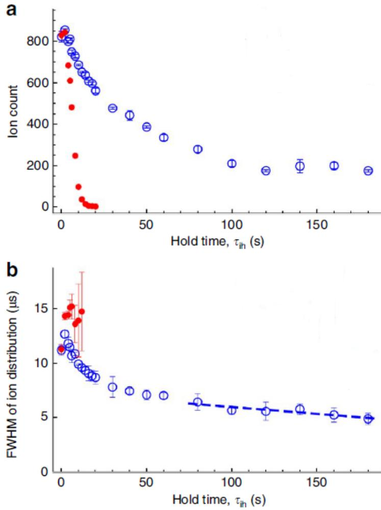
**Figure 4.10:** Change in the trapped ion population and the FWHM of ToF as a function of  $\tau_{ih}$  are plotted for ions held with cold atom (blue circles) and without cold atoms (red dots).
