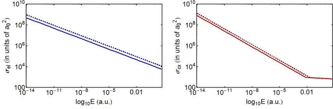
**Figure 5.6:** Elastic and charge exchange cross sections as a function of collision energy are illustrated in (a) and (b). Solid lines in both figures show the cross section values for the ground state, where  $C_4 = 5.26 \times 10^{-39} \text{Cm}^2/\text{V}$ . Dashed lines are for elastic and charge exchange cross section values in the excited state, where static polarizability is  $14.15 \times 10^{-39} \text{Cm}^2/\text{V}$ .
