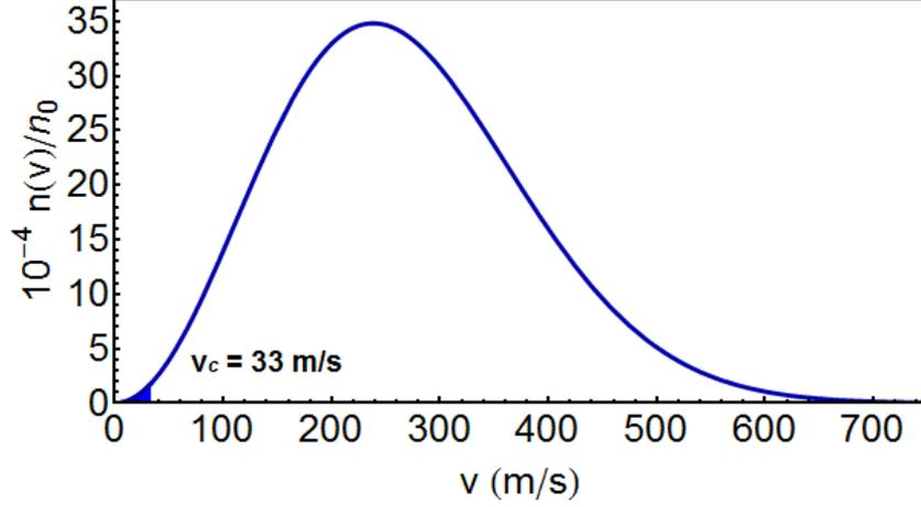
**Figure 3.9: Maxwell-Boltzmann distribution** of Rb vapour in room temperature of 293 K. Atoms with velocity less than the MOT capture velocity are indicated in the shaded region.
