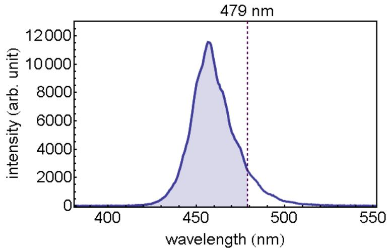
**Figure 3.19: Spectral profile of BLS:** The central wavelength of the BLS is at 456 nm and its  $\text{FWHM} = 22$  nm. Atoms require energy corresponding to 479 nm to get into ionization continuum. More than 90 % of the BLS spectrum participates in photo-ionization
