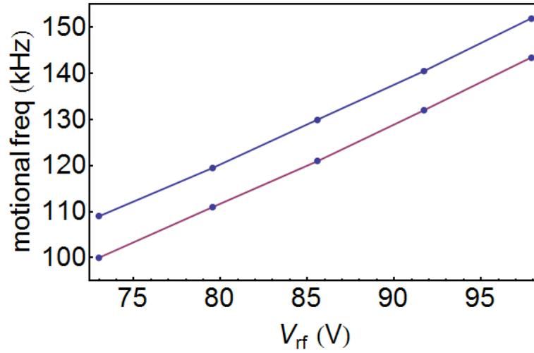
**Figure 3.25:**  $\omega_1$  (in red) and  $\omega_2$  (in blue) are plotted at various  $V_{rf}$  values. There is a prominent shift in resonances as  $V_{rf}$  value changes.
