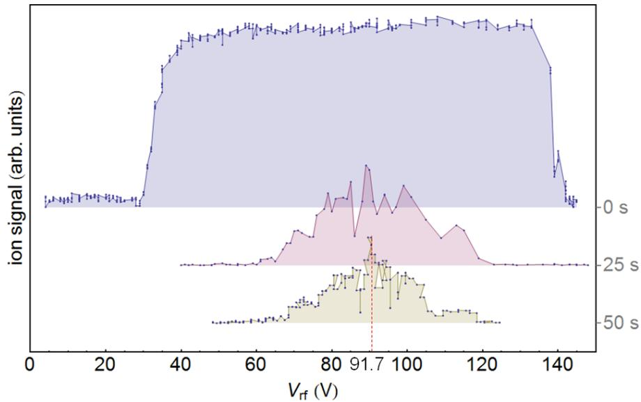
**Figure 3.26:** Stability region of the ions for 600 kHz scanned  $V_{rf}$  from 0 to 140 V for various holding times. Due to the gain-bandwidth limit of our RF amplifier, distortion in the drive voltage waveform starts from  $V_{rf} = 95$  V. For 50 s of holding time, the value of  $V_{rf}$  for the maximum number of ions detected is 91.7 V.
