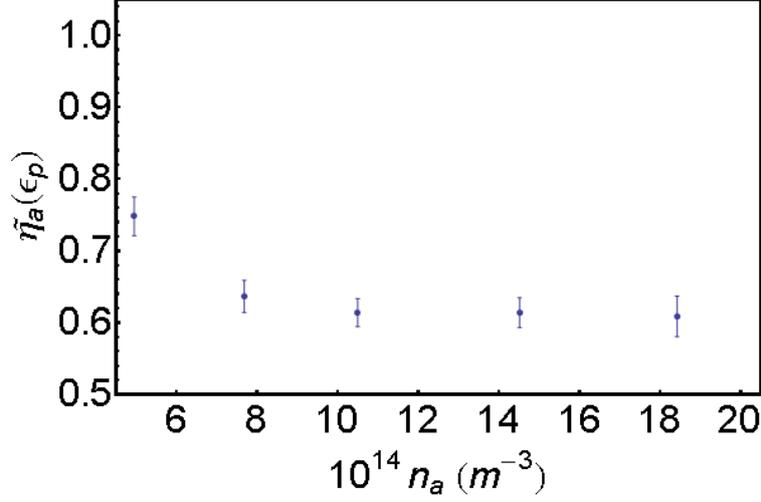
**Figure 3.32:** The change in MOT fluorescence  $\tilde{\eta}(\epsilon_p)$  is shown as a function of MOT density,  $n_a$ .  $\tilde{\eta}(\epsilon_p)$  remains constant  $n_a > 10 \times 10^{14} \text{ m}^{-3}$ .
