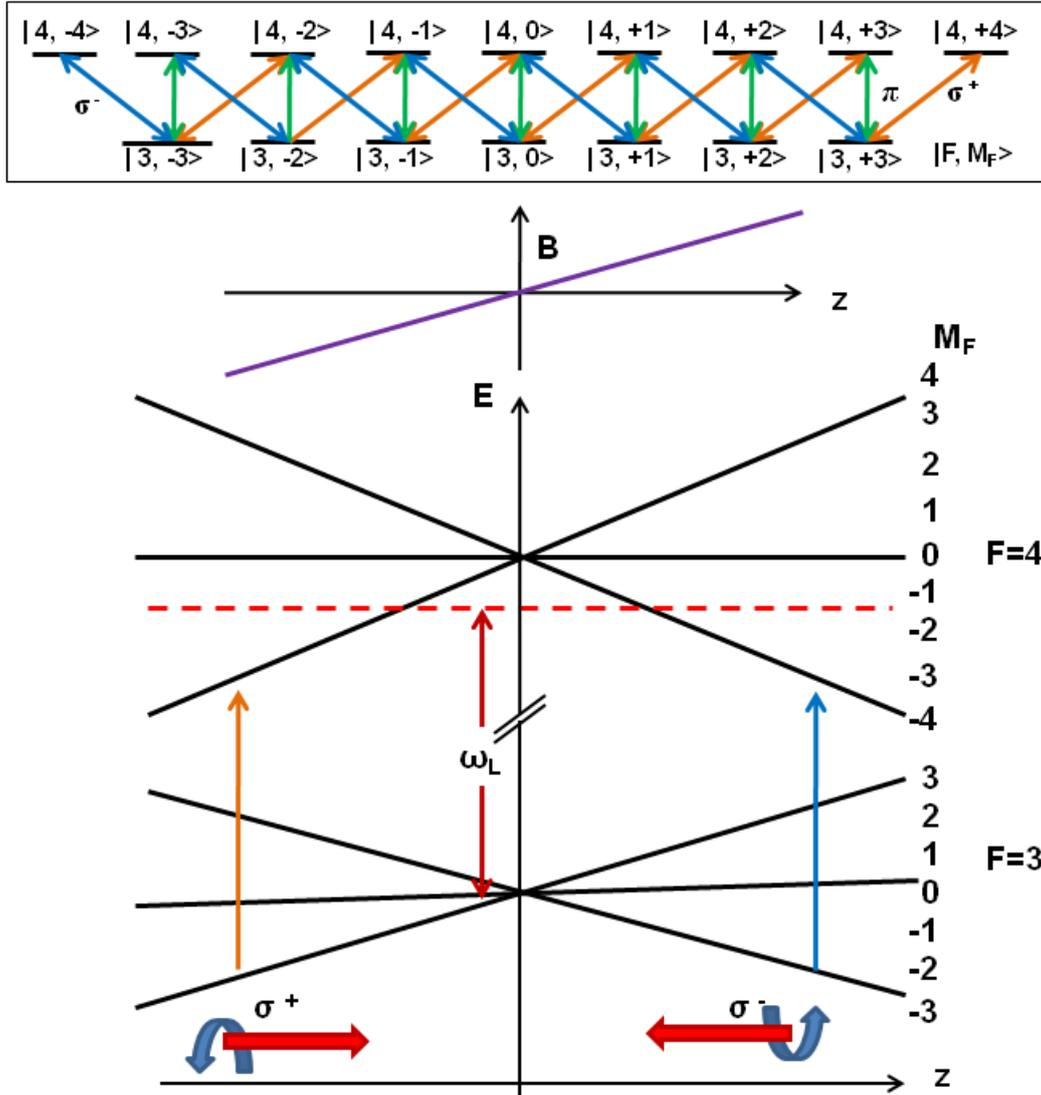
**Figure 3.2:** Fig. illustrates 1 D magnetic field ( $\mathbf{B}$ ) for MOT and simplified MOT scheme for  $|F = 3\rangle \rightarrow |F = 4\rangle$  transition. Inset shows the selective absorption of the circularly polarized light and magnetic sub levels for  $F = 3$  and  $F = 4$  (orange line indicates  $\sigma^+$  transition. Green line is for  $\pi$  transition and blue line is for  $\sigma^-$  transition).
