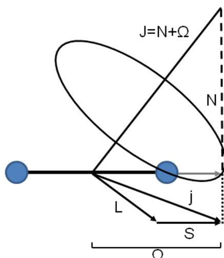
**Figure 3.28:** Vector coupling and projection for Hund's case c:  $\mathbf{j} = \mathbf{L} + \mathbf{S}$  is coupled to the internuclear axis. The projection of  $\mathbf{j}$  on the internuclear axis is  $\Omega$ , which is a good quantum number in Hund's case c.
