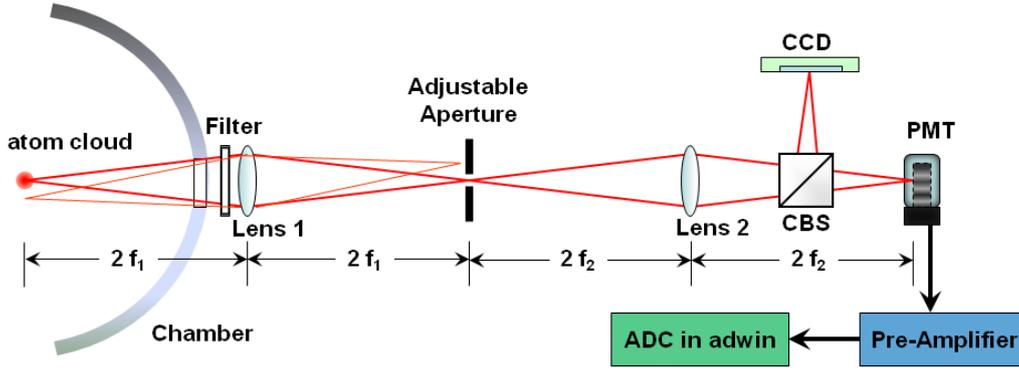
**Figure 3.11: Spatial filtering set up:** An illustration of the spatial filtering and imaging of the fluorescence from the MOT onto a PMT and CCD.
