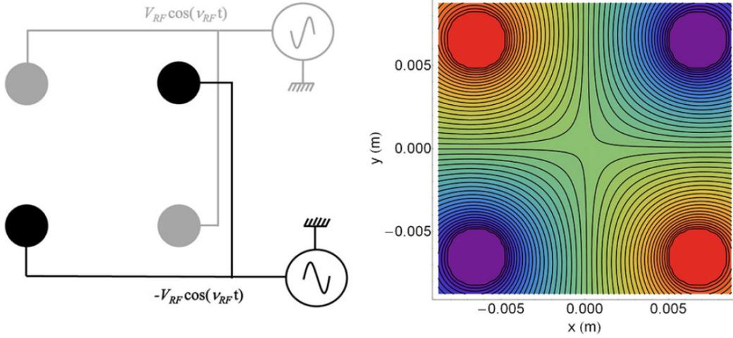
**Figure 3.17:** The cross section of the ion trap with the biasing diagram is illustrated. For a given instant of time, the resultant potential surface is plotted.
