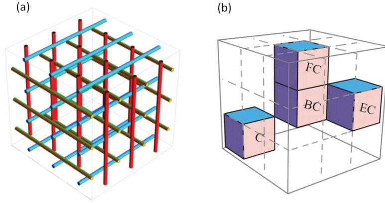
**Figure 2.2:  $3 \times 3 \times 3$  lattice of ion traps:** (a) illustrates the extension of the trap in 2.1 (a) to 27 LIT in a simple cubic arrangement. (b) Four distinct types of coordination symmetries for traps at different locations: Representative cells of different coordinations are identified as BC(6), FC(5), EC(4), and C(3), where the number of location-dependent nearest-neighbor cells is given in parentheses.
