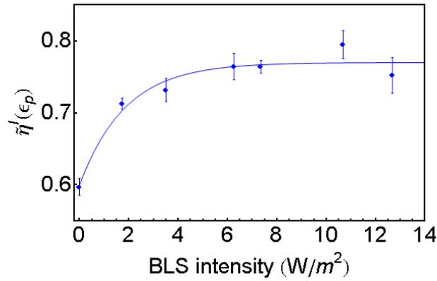
**Figure 6.3:** Figure shows the fractional increase in MOT fluorescence at  $\epsilon_p$  as a function of BLS intensity, which is proportional to ion loading rate into the ion trap.
