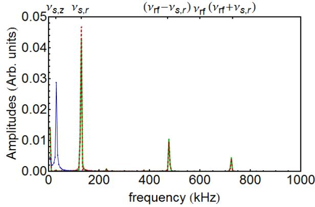
**Figure 4.6:** Fourier spectra of ion trajectories computed at  $\nu_{rf} = 600$  kHz in  $x$  (red, dashed),  $y$  (green) and  $z$  (blue) directions are illustrated. Fourier transform of each trajectory gives secular motion frequency,  $\nu_s$  of each direction.
