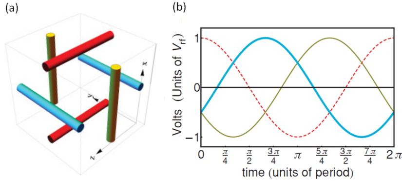
**Figure 2.1: Basic electrode configuration:** (a) Basic electrode configuration of the ion trap: three pairs of parallel electrodes are arranged along the Cartesian axes and are electrically contacted. (b) The relative phase difference of  $2\pi/3$  between the orthogonal electrode sets, where RF voltage applied along  $\hat{x}$ ,  $\hat{y}$  and  $\hat{z}$  are represented by thin, thick, and dashed lines, respectively.
