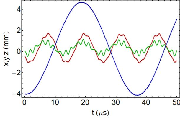
**Figure 4.5:** Trajectories of an ion in  $x$  (red),  $y$  (green) and  $z$  (blue) directions are calculated by MD simulation. Spatial extent of  $z$  trajectory is much larger than that of  $x$  and  $y$  due to the trap geometry and operation.
