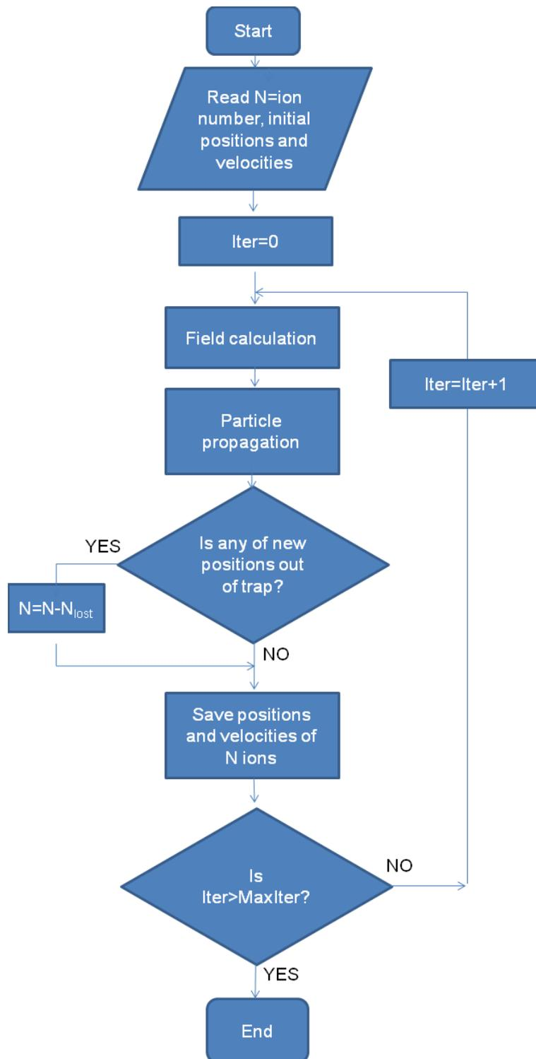
Figure 4.1: A flow chart for ion trajectory integration
