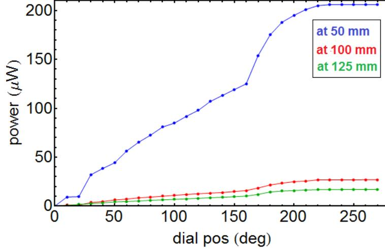
**Figure 3.20: Intensity of BLS as a function of dial position:** Intensity of BLS is measured at various distances, 50, 100 and 125 mm from the BLS.
