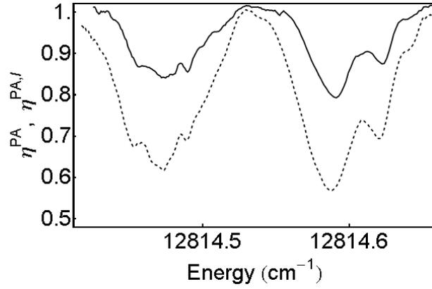
**Figure 6.2:** Figure illustrates the change in the fraction of MOT atoms lost due to PA as a function of PA laser frequency in the presence and absence of trapped ions, shown in blue ( $N_{pa} / N_{at}$ ) and dashed ( $N_{pa}^I / N_{at}^I$ ) lines respectively.
