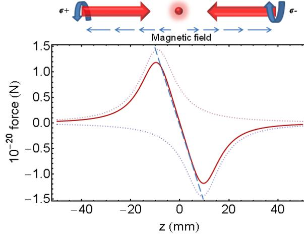
**Figure 3.3: Position dependent force for an one-dimensional magneto-optical trap :** Figure illustrates the scattering force as a function of position (solid lines) for a  $^{85}\text{Rb}$  atom in optical molasses with quadrupole magnetic field, where  $I = 3.5 \text{ mW/cm}^2$  per beam,  $\delta = 15 \text{ MHz}$  and  $\frac{dB}{dz} = 12 \text{ G/cm}$ . The forces produced by each counter propagating laser beams are plotted as dotted lines.
