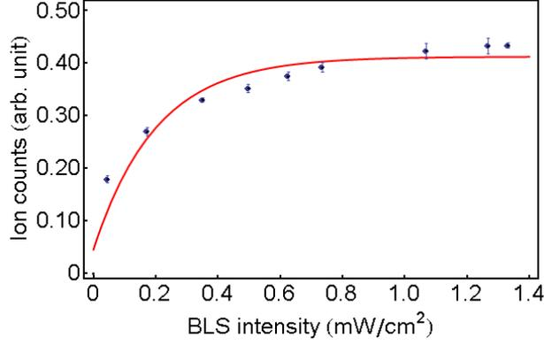
**Figure 5.5:** (color online) The change in the detected ion counts vs. BLS intensity is shown. Since the number of trapped ions is very large, severe pileup of the ion signal results and the ion signal is seen to saturate faster than measured from the atom signal. The fit is generated using Eq. (5.15).
