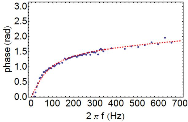
**Figure 3.15:** Figure illustrates the frequency response of the phase of the atom cloud motion when subjected to a sinusoidal perturbation which is fitted to Eq. 3.16. The fit yields  $\kappa_{MOT} = 1.695 \times 10^{-20} \text{ kg/s}^2$  and  $c = 2m_{Ap} = 2.541 \times 10^{-22} \text{ kg/s}$ .
