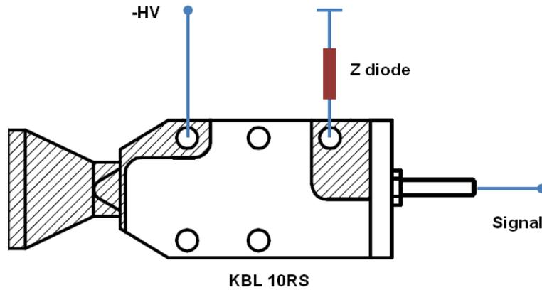
**Figure 3.21: CEM connection:** Zener diode is used for creating a stable voltage difference about 100 V between the CEM output and the anode. The diagram is taken from sjuts.com.
