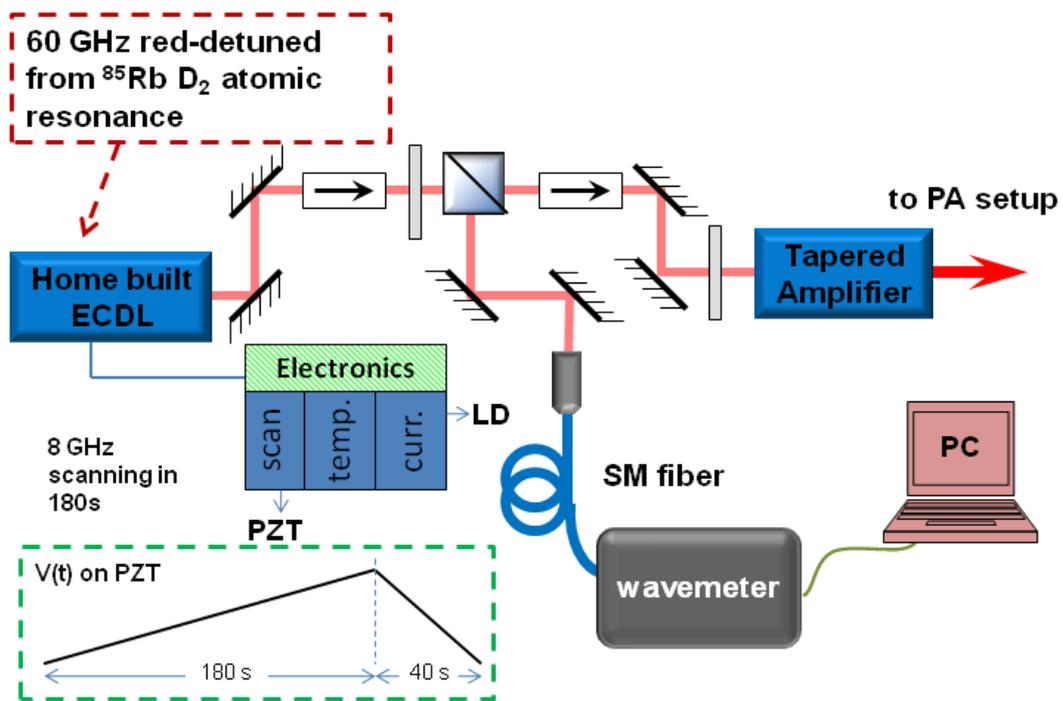
**Figure 3.30:** For PA, a home-built ECDL is adjusted to give 60 GHz red-detuned from  $^{85}\text{Rb D}_2$  transition. Using a scan-controller from toptica, we can scan over 8 GHz at 44 MHz/s speed. A small part of the laser light is fed to the wavemeter to monitor the scanning frequency. Rest of all the light is then fed to a tapered amplifier for intensity amplification.
