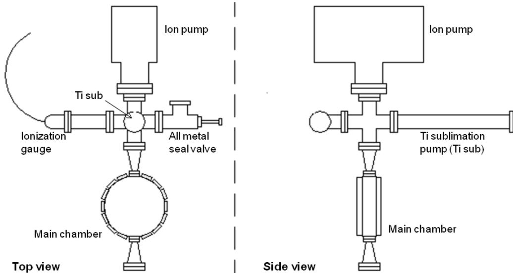
**Figure 3.7: UHV system geometry:** A simple outline diagram of the vacuum chamber with ion pump (constantly in operation) and titanium sublimation pump. The pressure inside is measured using an ionization gauge.
