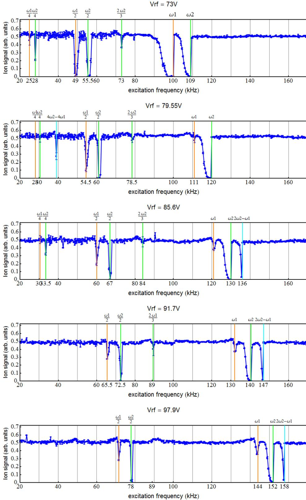
**Figure 3.24:** The spectra of motional resonances of a  $\text{Rb}^+$  ion cloud in the trap at  $V_{rf} = 73, 79.55, 85.6, 91.7$  and  $97.9$  V.  $\omega_1$  and  $\omega_2$  are radial resonance frequencies. Other than  $\omega_1$  and  $\omega_2$ , we also observe higher harmonics of resonance frequencies.
