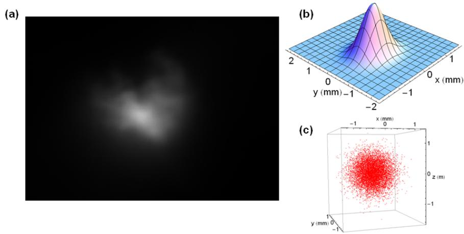
**Figure 3.12: Density profile of Rb atoms in the MOT:** (a) illustrates an image of the fluorescence from atom cloud in the MOT, captured on a CCD camera in the spatial filtering setup. Data from the captured image in (a) is fitted to a Gaussian distribution. The spatial profile of the atom cloud is shown in (b). The rms size of the atom cloud is found to be  $\approx 0.35$  mm. (c) shows simulated atom cloud of Gaussian distribution with  $\sigma = 0.35$  mm.
