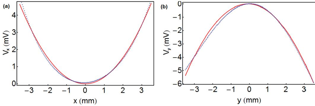
**Figure 3.18:** A fit of Eq. 3.26 to the central portion of the SIMION generated potential is illustrated. (a) plots  $V_x = V(x, y = 0, t = 0)$  and (b) plots  $V_y = V(x = 0, y, t = 0)$ .
