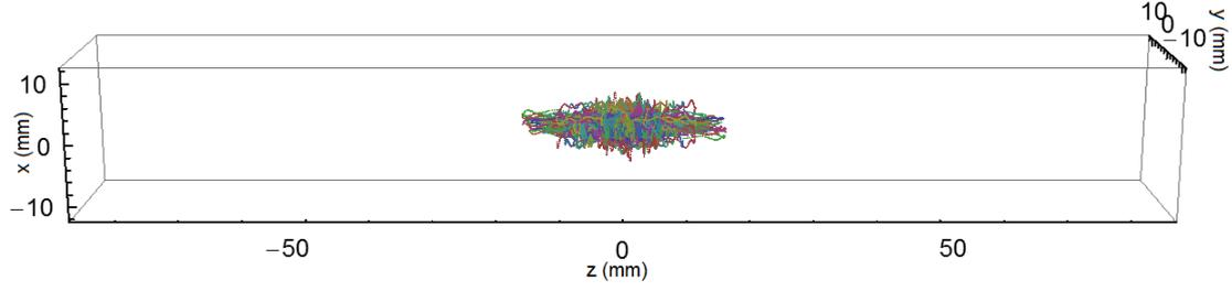
**Figure 4.7:** About 200 ions are evolved in the ion trap for  $50 \mu\text{s}$ . Ion cloud has an ellipsoidal shape of  $r_x = r_y < r_z$ .
