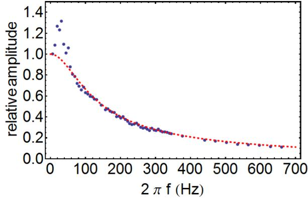
**Figure 3.14:** The frequency response of the relative amplitude of the atom cloud motion is illustrated when subjected to a sinusoidal perturbation. A red dashed line is a fit using Eq. 3.15 yielding  $\kappa_{MOT} = 1.695 \times 10^{-20} \text{ kg/s}^2$  and  $c = 2m_{Ap} = 2.027 \times 10^{-22} \text{ kg/s}$ .
