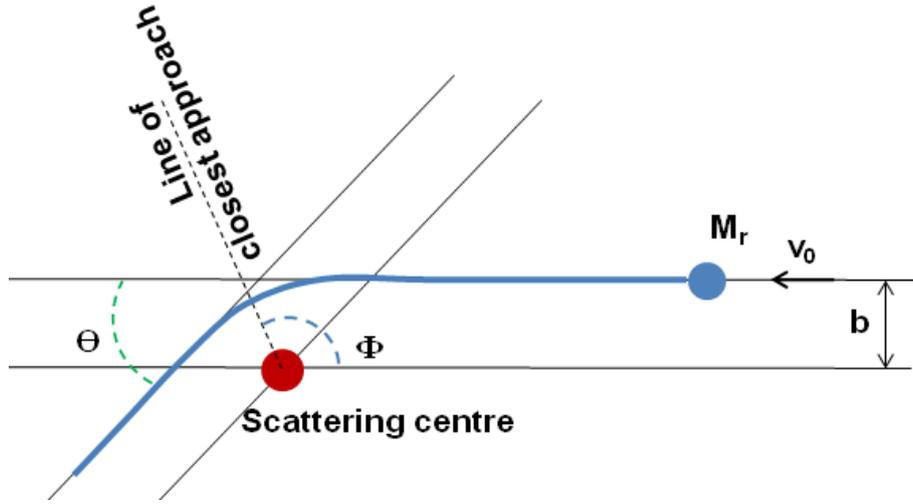
**Figure C.1:** The one body scattering, dynamically equivalent to the two body scattering is illustrated.  $M_r$  is scattered through an angle,  $\Theta$  whose value is calculated in Eq. C.2.
