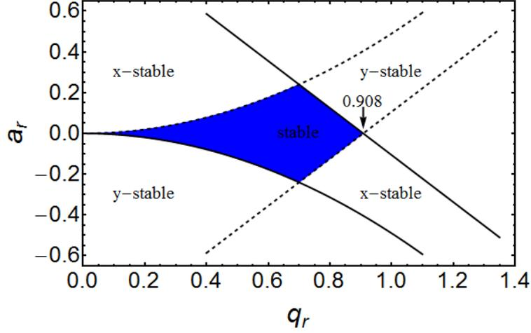
**Figure 2.3:** The first stability region in the radial direction for a linear Paul trap.  $q$  ranges from 0 to 0.908 for  $a = 0$ .
