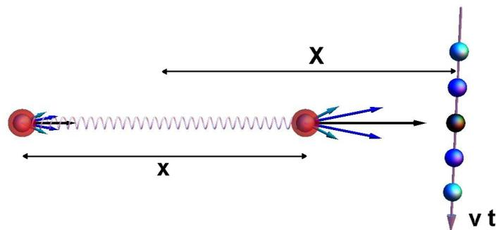
**Figure 6.4:** Toy model figure shows the effect of the passage of the ion in the vicinity of the molecule. The two atoms experience a different forces as they polarize independently under the influence of the ion. This results in an overall differential force along the molecular bond, which enables vibrational excitation of the molecule.
