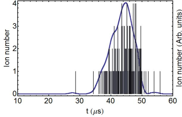
**Figure 4.9:** Left-side y axis shows ToF analysis of the ion arrival times at the CEM's position and right-side y axis is the convoluted arrival times distribution of ions with the preamplifier response function.
