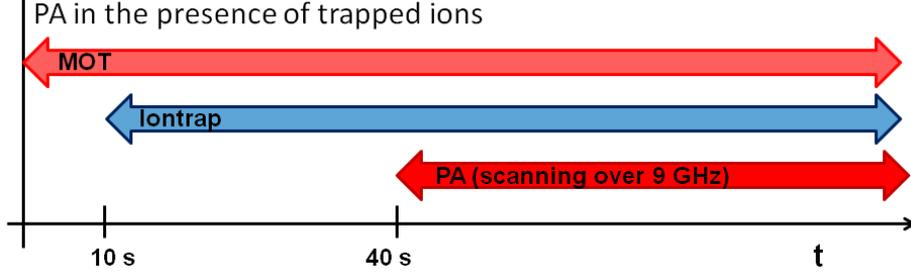
**Figure 6.1:** Experimental sequence of PA experiment in the presence of trapped ions is illustrated. Once MOT reaches its saturation at  $t = 10$  s, the BLS and iontrap are switched on simultaneously to trap ions. At  $t = 30$  s, MOT and iontrap both reach a steady state. Then PA laser scans over  $\approx 9$  GHz.
