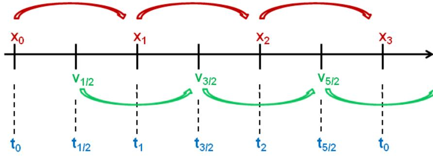
**Figure 4.3:** This method uses the derivatives at the midpoint of each step. This only requires one additional step to be taken in order to move the velocity a half step ahead of the position. Because of its better accuracy while still keeping the computation time relatively low, the Leapfrog method is employed in the simulation.
