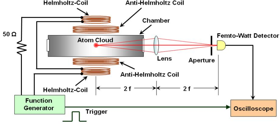
**Figure 3.13: Experimental set up for MOT temperature measurement:** An illustration of the spatial filtering and imaging of the fluorescence from the MOT onto a femto-watt detector.
