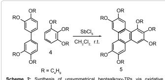
**Scheme 2:** Synthesis of unsymmetrical heptaalkoxy-TPs via oxidative coupling of a 1,2,3-trialkoxybenzene with a tetraalkoxybiphenyl.
