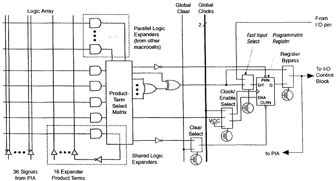
Figure 4 shows a MAX 7000E and MAX 7000S device macrocell.
