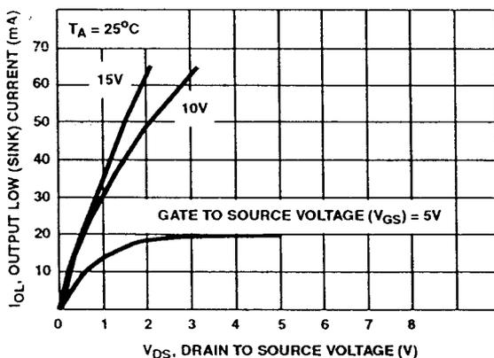
FIGURE 4. TYPICAL OUTPUT LOW (SINK) CURRENT CHARACTERISTICS
