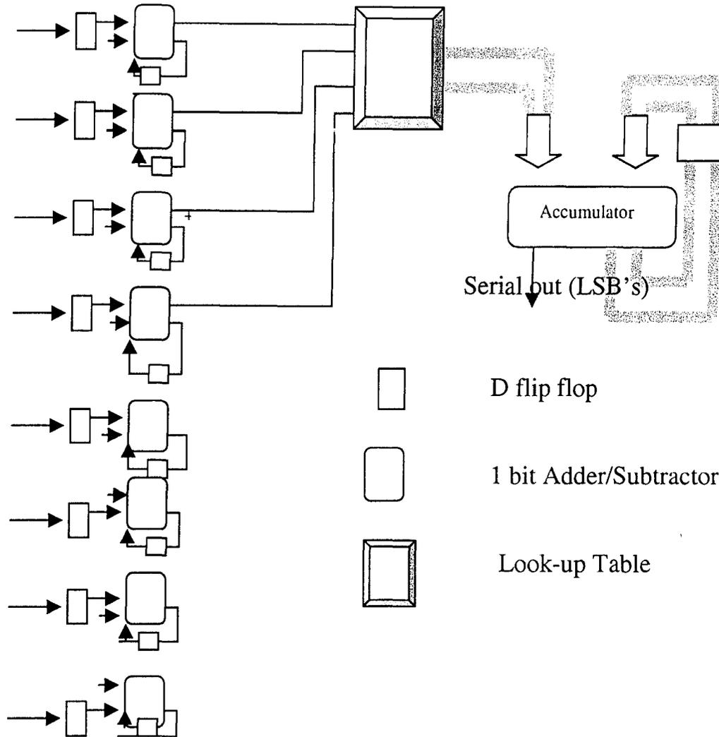
Fig.3.5 Block diagram of 1-D DCT implemented using the ROM-Accumulator module and the Decomposition approach.
