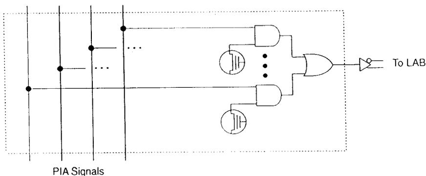
While the routing delays of channel-based routing schemes in masked or FPGAs are cumulative, variable, and path-dependent, the MAX 7000 PIA has a fixed delay. The PIA thus eliminates skew between signals and makes timing performance easy to predict.
