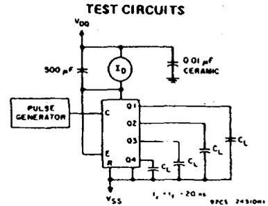
Fig. 10 - Dynamic power dissipation.
