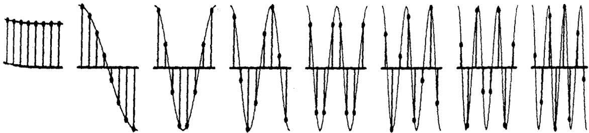
**Fig.1.4.** *Basis functions for the Discrete Cosine Transform*
