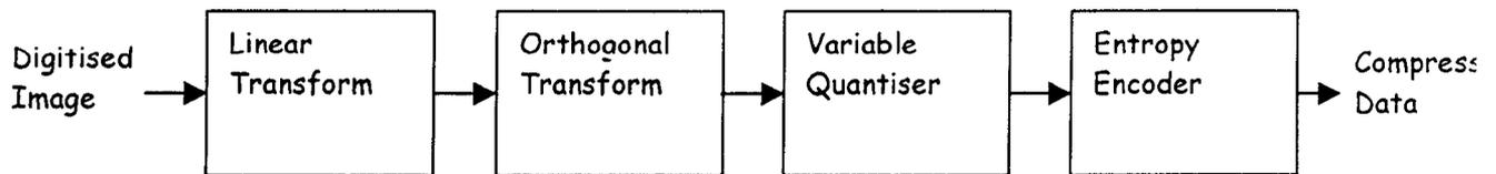
**Fig.1.2** Block diagram of general image compression system
