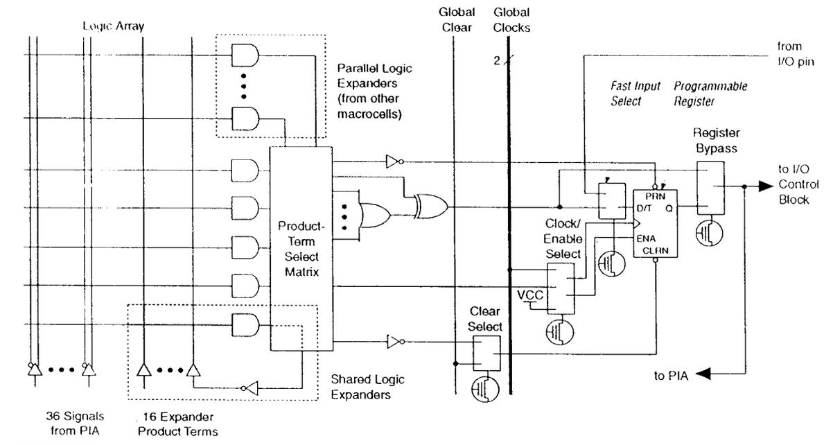
Combinatorial logic is implemented in the logic array, which provides five product terms per macrocell. The product-term select matrix allocates these product terms for use as either primary logic inputs (to the OR and XOR gates) to implement combinatorial functions, or as secondary inputs to the macrocell's register clear, preset, clock, and clock enable control functions. Two kinds of expander product terms ("expanders") are available to supplement macrocell logic resources:
