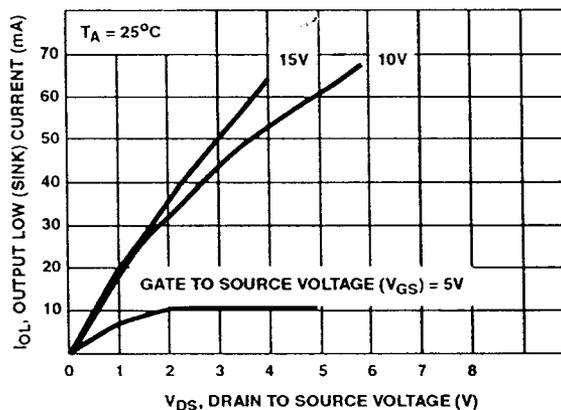
FIGURE 5. MINIMUM OUTPUT LOW (SINK) CURRENT DRAIN CHARACTERISTICS
