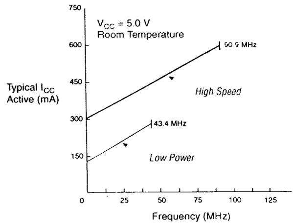
Figure 15 shows typical supply current versus frequency for MAX 7000S devices.
