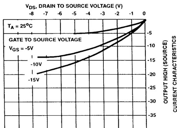
FIGURE 7. MINIMUM OUTPUT HIGH (SOURCE) CURRENT CHARACTERISTICS
