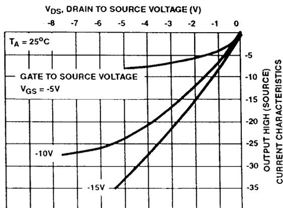
FIGURE 6. TYPICAL OUTPUT HIGH (SOURCE) CURRENT CHARACTERISTICS
