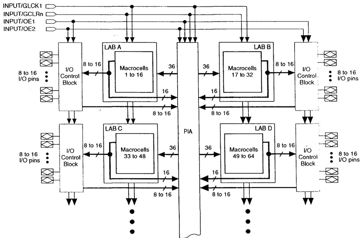
Figure 1 shows the architecture of MAX 7000E and MAX 7000S devices.
