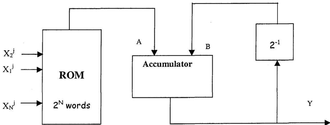
*Fig.3.4 ROM-Accumulator unit for the implementation of sum of products using Distributed Arithmetic*
