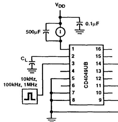
$C_L$  INCLUDES FIXTURE CAPACITANCE
