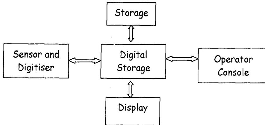
**Fig 1.1** *General purpose Image Processing System*
