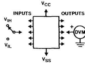
NOTE: Test any one input with other inputs at  $V_{CC}$  or  $V_{SS}$ .
