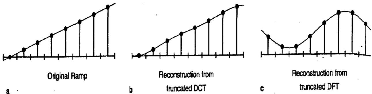
**Fig.1.5.** A comparison of the accuracy of the truncated & reconstructed DCT and DFT for the ramp signal
