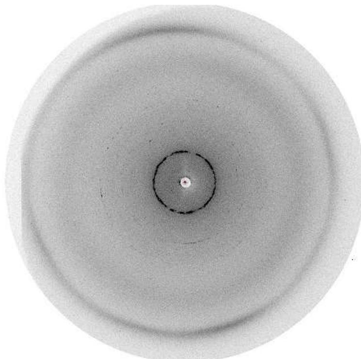
**Figure 10.** X-ray diffraction pattern of the compound **15a** in the mesophase.
