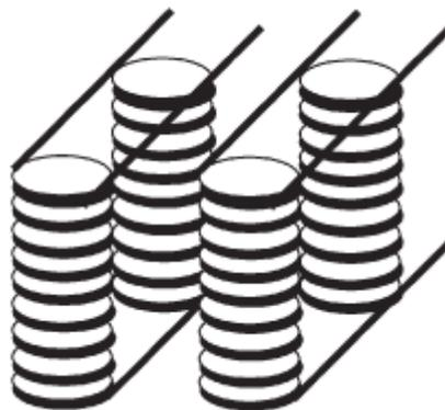
**Figure 22.** Columnar lamellar phase.
