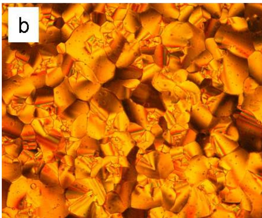
**Figure 18.** Optical photomicrograph of (a) **10** and (b) composite **10b** at 25 °C on cooling from the isotropic liquid (crossed polarizers, magnification X 200).
