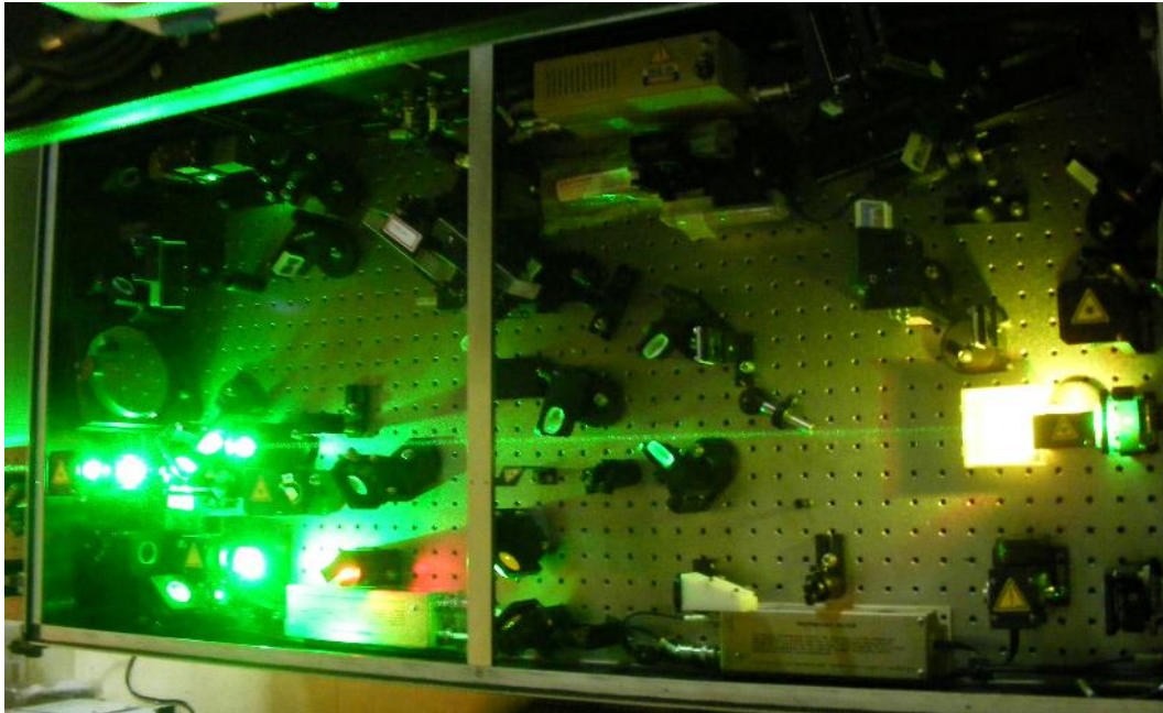
Figure 5.3: The CPA system used for the experiments (view from above).
