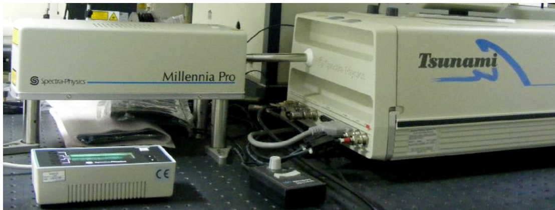
Figure 5.2: The Tsunami oscillator along with the Millennia pump laser.
