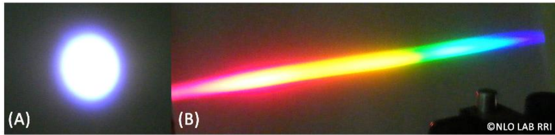
Figure 4.1: (A) White-light continuum generated in water using 800 nm, 100 fs laser pulses. (B) The continuum dispersed using a grating.
