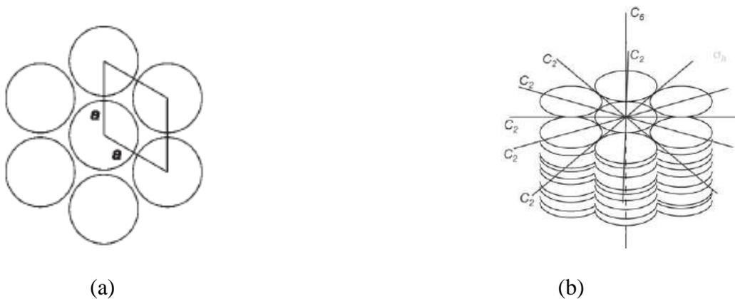
**Figure 12.** (a) Plan views of the 2D lattices in hexagonal (b) symmetry elements of a Col<sub>h</sub> mesophase: the point group  $D_{6h}$  has one  $C_6$  axis and perpendicular to this axis, six  $C_2$  and a mirror plane  $\sigma_h$ .
