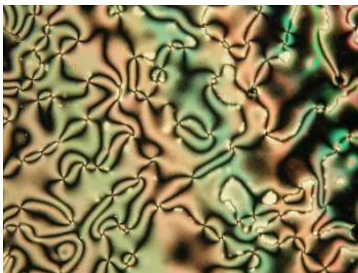
Figure 16. Optical photomicrograph of compound 15c on cooling the isotropic liquid at 100\text{ }^{\circ}\text{C} (crossed polarizers, magnification X 200).
