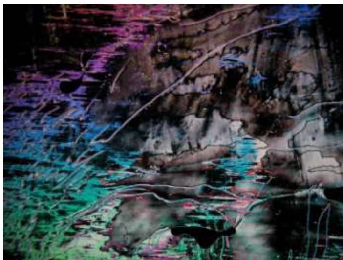
Figure 19. Optical texture of the nematic phase of dimer 15e obtained on cooling from the isotropic liquid at 105 °C (crossed polarizers, magnification X 200).
