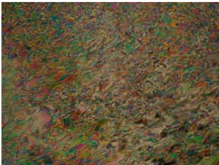
Figure 17. Optical photomicrograph of compound 28c at 90 °C on cooling from isotropic liquid (Crossed polarizers, magnification X 200).
