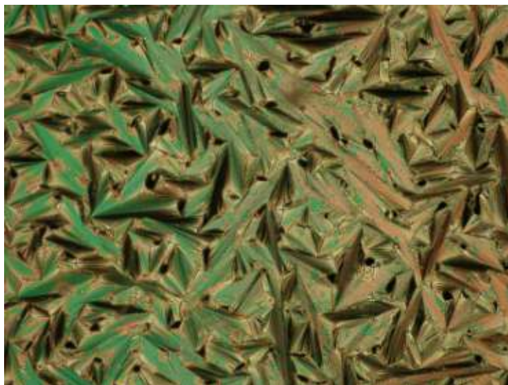
Figure 33. Optical texture of compound 24c obtained on cooling from the isotropic liquid at 120 °C (crossed polarizers, magnification X 200).
