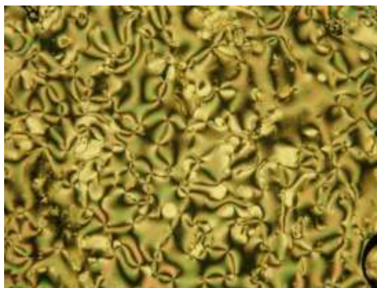
Figure 30. Optical texture of compound 24a obtained on cooling from the isotropic liquid at 170 °C (crossed polarizers, magnification X 200).
