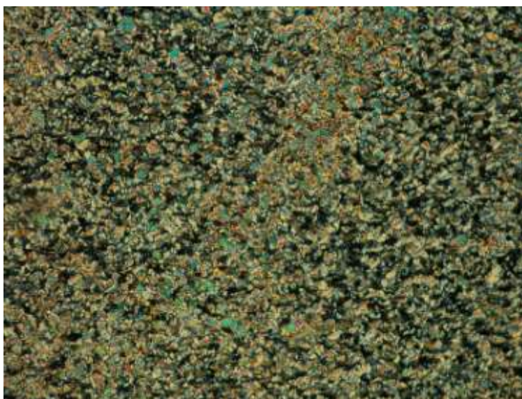
Figure 7. Optical Photomicrograph of compound 18a obtained on cooling from the isotropic liquid at 35 °C (crossed polarizers, magnification X 200).
