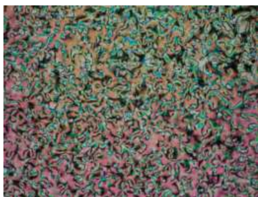
Figure 30. Optical texture of compound 24a obtained on cooling from the isotropic liquid at 170 °C (crossed polarizers, magnification X 200).
