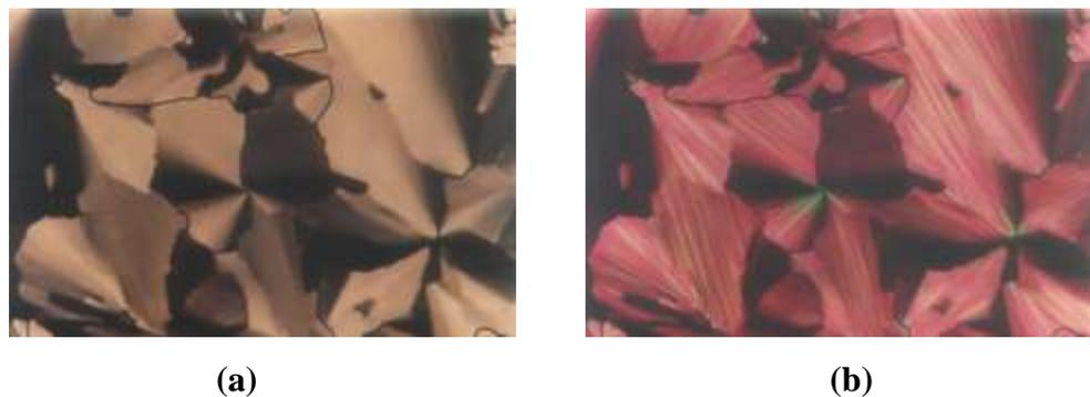
**Figure 3.11: Textures of compound 3.B.6 obtained under triangular-wave field, T=135°C.
