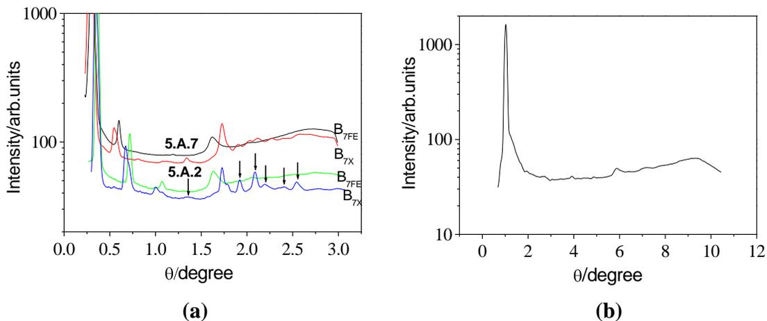
**Figure 5.9:** Plots of intensity *versus* Bragg angle ( $\theta$ ) obtained from the X-ray diffraction pattern. (a) Compound 5.A.2 at  $T=150^\circ\text{C}$  ( $B_{7FE}$ ),  $130^\circ\text{C}$  ( $B_{7X}$ ) and compound 5.A.7 at  $T=140^\circ\text{C}$  ( $B_{7FE}$ ),  $112^\circ\text{C}$  ( $B_{7X}$ ); (b) compound 5.B.6 at  $T=120^\circ\text{C}$  ( $B_{7FE}$ ).
