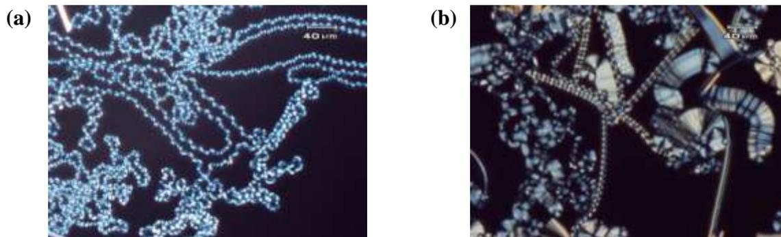
**Figure 5.5: Textural photomicrographs obtained for the B<sub>7FE</sub> phase of compound 5.A.7 in two different regions of the same sample, T=165°C.**
