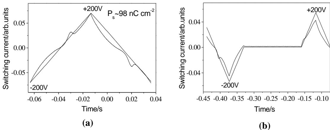
**Figure 5.10:** Switching current response trace obtained for the  $B_{7FE}$  phase of compound 5.A.7 at  $140^\circ\text{C}$  in an ITO coated cell of thickness  $13.4 \mu\text{m}$  by applying (a) triangular-wave voltage,  $400V_{pp}$ , 10Hz and (b) modified triangular-wave voltage,  $400V_{pp}$ , 4Hz.
