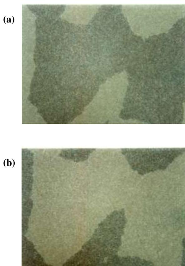
**Figure 5.15: Microscopic texture of the B<sub>7</sub> phase of compound 5.D.2 obtained on rotating the polarizer by a) +5° and b) -5° from its crossed position, T=140°C.**
