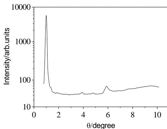
**Figure 5.18: X-Ray angular intensity profile obtained for the B<sub>7</sub> mesophase of compound 5.D.4, T=135 $^{\circ}\text{C}$ .**
