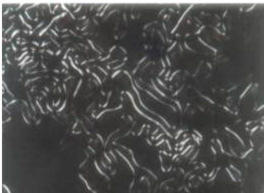
**Figure 5.16: Photomicrograph showing the filamentary texture for the B<sub>7</sub> phase of compound 5.D.4, T=141.5°C.**
