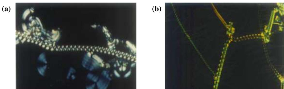
**Figure 5.12: (a) and (b), Photomicrographs of the helical patterns forming on cooling the isotropic phase of compound 5.C.4,  $T=145.5^{\circ}C$ .**
