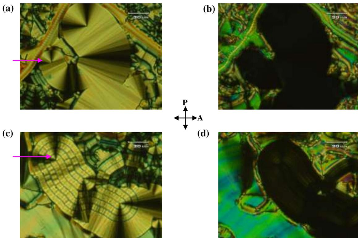
**Figure 5.6: Photomicrographs obtained for compound 5.A.7 showing the textural change after the phase transition  $B_{7FE} \rightarrow B_{7X}$  in a cell of thickness  $5 \mu\text{m}$  treated for planar alignment; (a) and (c) at  $T=150^\circ\text{C}$ ; (b) and (d) at  $T=115^\circ\text{C}$  (same region as in a and c respectively).**
