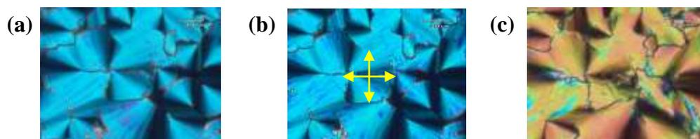
**Figure 5.11: Photomicrographs obtained for the mesophase of compound 5.A.7 on application of triangular-wave electric field. (a)  $400V_{pp}$ , 10Hz,  $140^\circ\text{C}$ ; (b) on switching off the field,  $140^\circ\text{C}$ ; (c)  $400V_{pp}$ , 10 Hz,  $120^\circ\text{C}$ .**
