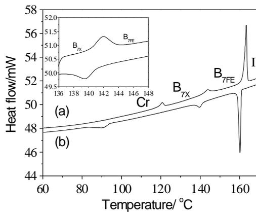
**Figure 5.3:** A DSC thermogram obtained for compound 5.A.2 at a scan rate of  $5^{\circ}\text{C min}^{-1}$ ; (a) heating cycle; (b) cooling cycle. The inset shows an enlarged view of the mesophase to mesophase transition (scan rate  $0.1^{\circ}\text{C}$ ).
