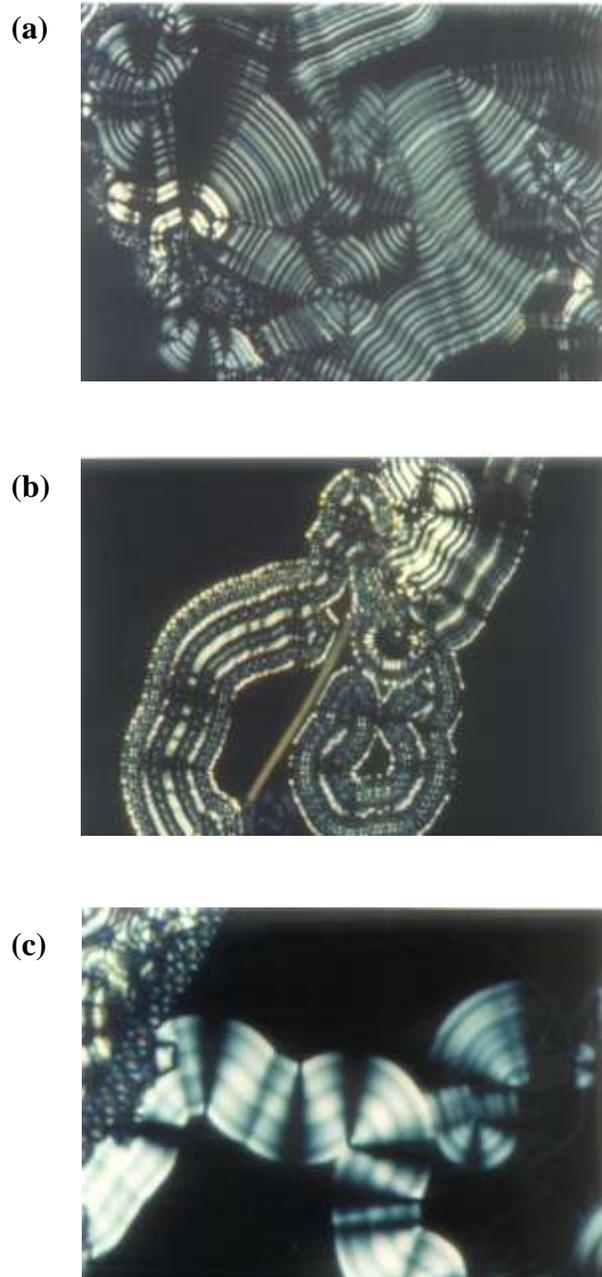
**Figure 5.13: (a), (b) and (c), Various fascinating patterns of the B<sub>7</sub> phase of compound 5.C.4 obtained on slow cooling of the isotropic phase, T=145.5°C.**
