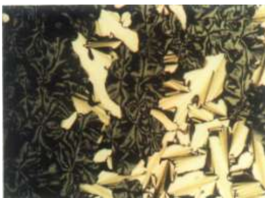
Figure 6.1: Photomicrograph of the texture obtained for the mesophase of compound 6.A.6, T=110°C.
