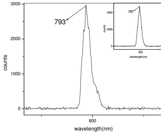
Figure 5.5: Doppler shifted fundamental frequency. A blue shift of 4nm is observed in the fundamental that is reflected at  $45^\circ$  from the plasma. Here the input is *p*-polarized. Inset shows the spectrum of the original laser pulse.
