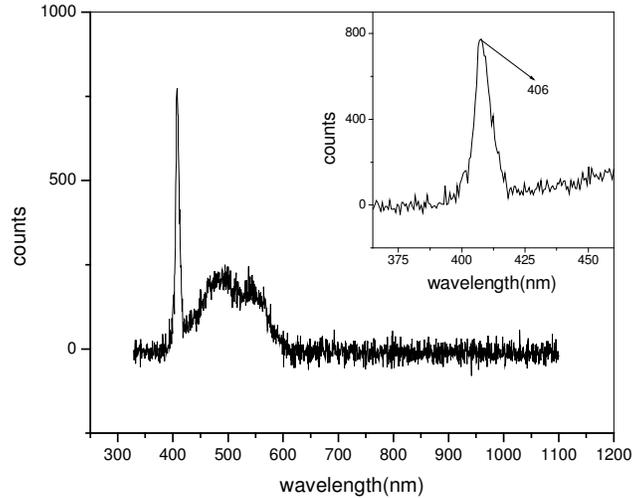
Figure 5.6: SH emission observed at the  $45^0$  specular reflection direction. An expanded SH is shown in the inset. The peak is at 406nm for this  $p$ -polarized incidence.
