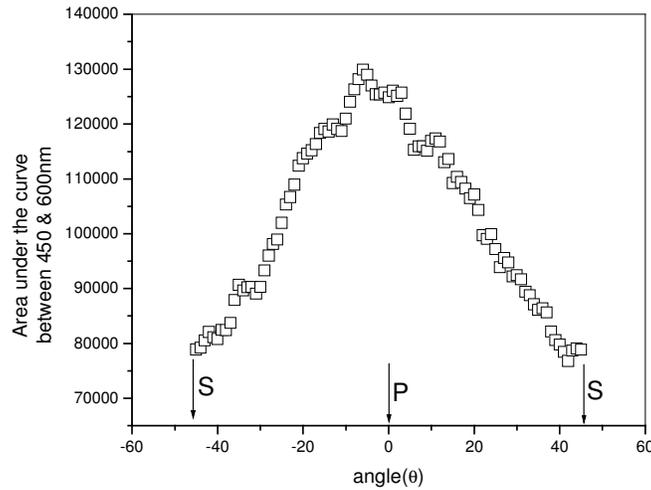
Figure 5.3: Area under the curve for emission between 450 nm and 600 nm (incoherent white light emission) observed in the specular reflection direction.
