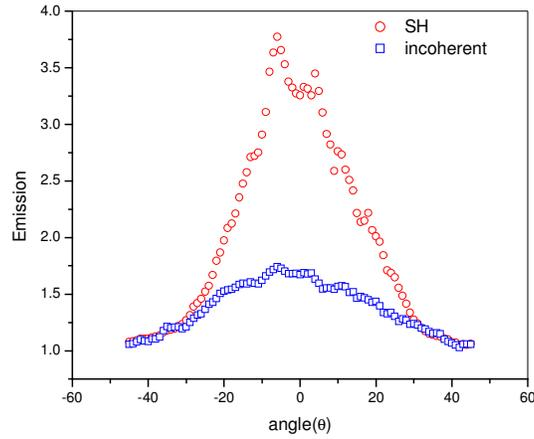
Figure 5.4: Plot of SH emission and incoherent emission. The emission intensities are normalized to a value of 1 for *s*-polarized input.
