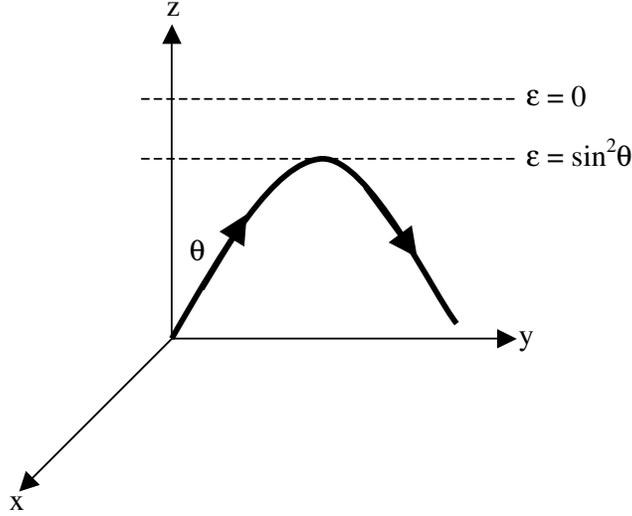
Figure 5.1: Light ray obliquely incident on an inhomogeneous plasma slab
