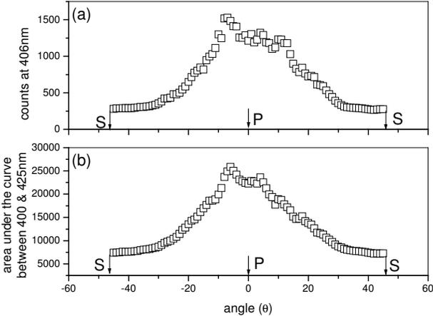
Figure 5.2: (a) Intensity of SH emission at 406nm plotted as a function of the input laser polarization.  $0^\circ$  corresponds to  $p$ -polarized state of the input laser. (b) Area under the curve measured for emission between 400 and 425 nm.
