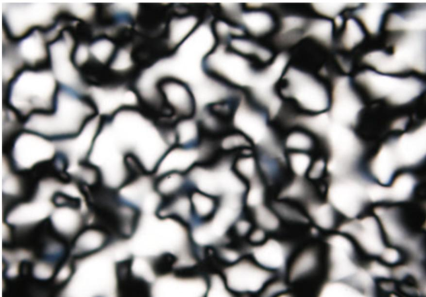
Figure 2.8: A polarizing microscope image of CSPFO water system in the nematic ( $N_D$ ) phase showing a schlieren texture. The magnification was  $200\times$  and sample was kept between crossed polarizers.
