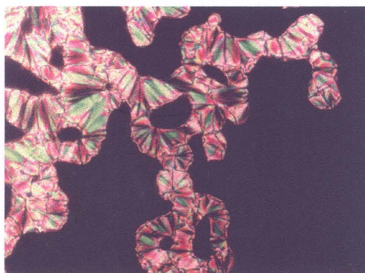
Figure 4.1: An optical photomicrograph of SmCP A phase growing from isotropic phase of compound 4.A.3.
