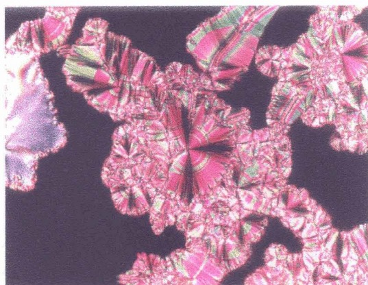
Figure 4.7: An optical photomicrograph of the fan-shaped texture obtained for compound 4.B.8.
