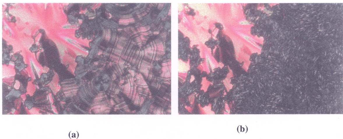
Figure 7.6: Optical photomicrographs obtained for the B 2 mesophase of compound 7.A.3 (a) with the electric field; (b) without the electric field.
