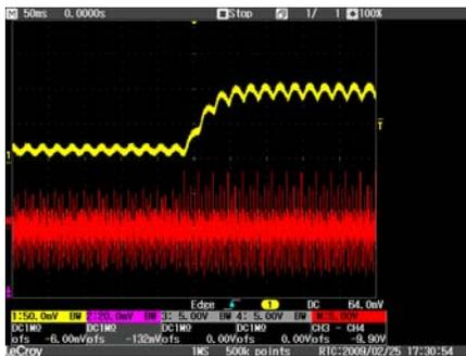
**Figure 1** Transmission of light through a pixel in a matrix LCD when the pixel is switched from one gray shade to another. Intensity of light falling on the detector to some extent follows the instantaneous voltage across the pixel; whereas the average light throughput depends on the RMS voltage.
