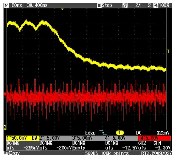
**Figure 4** Transmission of light through a pixel (yellow) when the scanning sequence is chosen to distribute all the select pulses in the addressing waveform (red).
