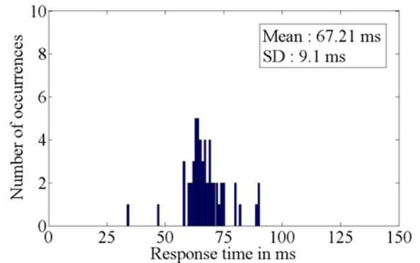
**Figure 8** Number of occurrences of response times when four select vectors and their rotated version are used to obtain the clustering of select pulses that are separated by applying non-select voltage during 112 time intervals.
