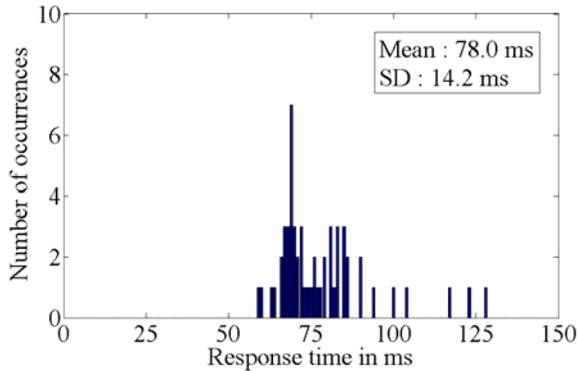
**Figure 5** Number of occurrences of response time vs response time in ms when the scanning sequence has 32-select pulses clustered.
