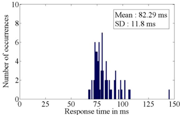
**Figure 10** Number of occurrences of response times vs. response times for successive approximation technique based on line-by-line addressing.
