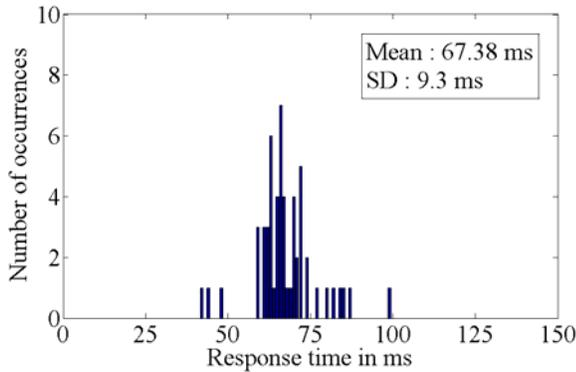
**Figure 9** Number of occurrences of response time vs. response time when rows are selected with the orthogonal matrix with 3 rows obtained by eliminating the zeros in (1). Here row waveforms have clusters of 12 select pulses.
