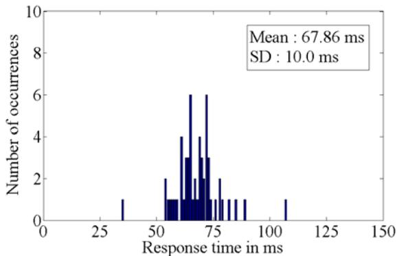
**Figure 6** Number of occurrences of response time vs. response time in ms when 4 select pulses i.e., elements of a column of a select vector are clustered and such clusters are separated by 28 time intervals of non-select voltage.
