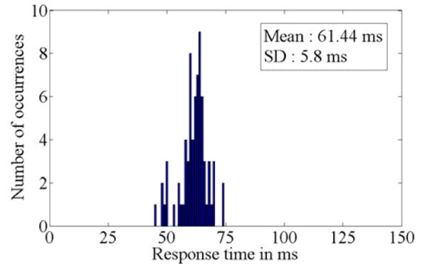
**Figure 11** Distribution of response times of multi-line addressing with sparse matrix by selecting seven rows simultaneously (for comparison)
