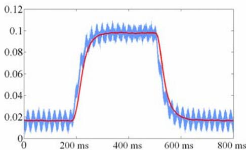
**Figure 2** Transmission of light through a pixel that is captured using a digital storage oscilloscope (blue) and the plot of response time after filtering (moving average of data captured during 20ms) is shown in red line.
