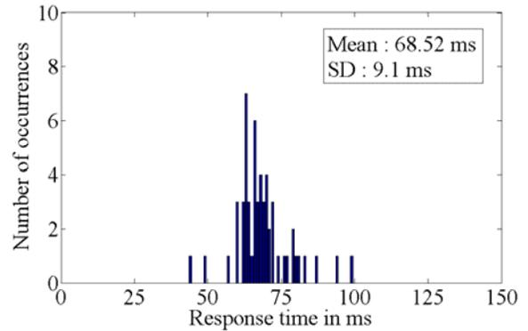
**Figure 7** Number of occurrences of response time vs. response time in ms when the cluster of scanning pulses are obtained with 2-select vectors wherein clusters are separated by 56 non-select time intervals.
