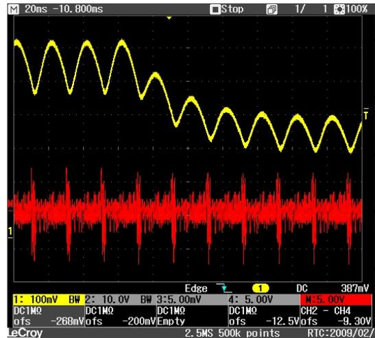
**Figure 3** Transmission of light through a pixel (yellow) when it is switched from one gray shade to another by using 32-select pulses that are clustered (red).
