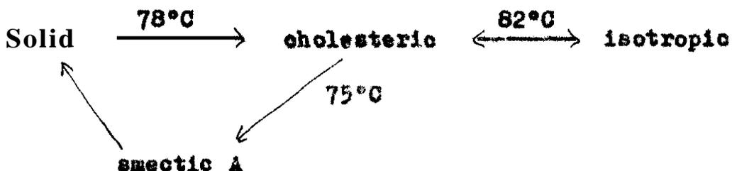
About 200–300 milligrams of **the** mixture was prepared in a **small** glass cup and it was heated in a oven to temperatures slightly above the cholesteric-isotropic **transition temperature**. It was stirred well with a **glass** rod to get homogeneous melt and then cooled to get the cholesteric phase,
