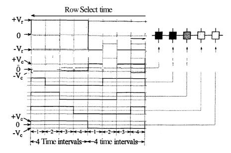
Figure 2-26 Gray shade generation using pulse width modulation method.
