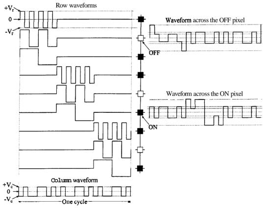
Figure 2-15 Typical addressing waveforms of HAT, for N = 9 and s = 3.
