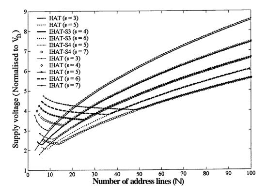
Figure 2-19 Supply voltage (Normalized to  $V_{th}$ ) versus number of address lines N for IHAT, HAT, IHAT-S3 and IHAT-S4.
