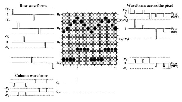
Figure 2-36 Typical addressing waveforms of RPAT-PC, displaying two waveforms.
