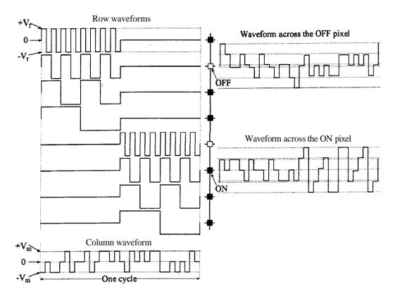
Figure 2-16 Typical addressing waveforms of IHAT-S3, for N = 8 and s = 4.
