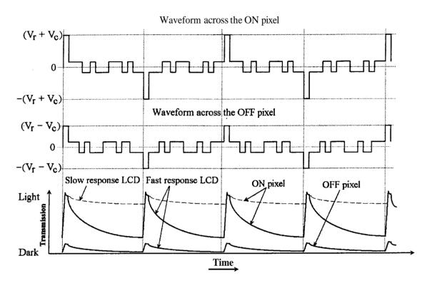
Figure 2-10 Frame response phenomenon in line by line addressing.
