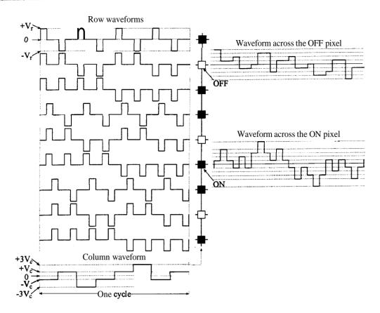
Figure 2-13 Typical addressing waveforms of IHAT (N = 9 and s = 3), row select pulses are distributed in a cycle.
