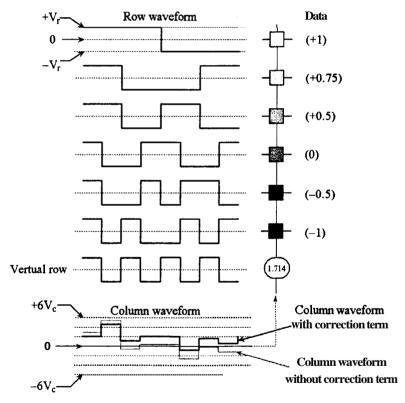
Figure 2-31 Typical addressing waveforms of active addressing amplitude modulation technique for displaying gray shades.
