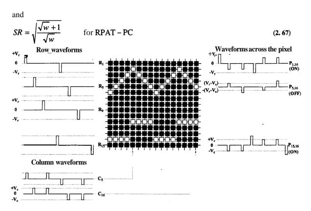
Figure 2-35 Typical addressing waveforms of RPAT-NC, displaying two waveforms.
