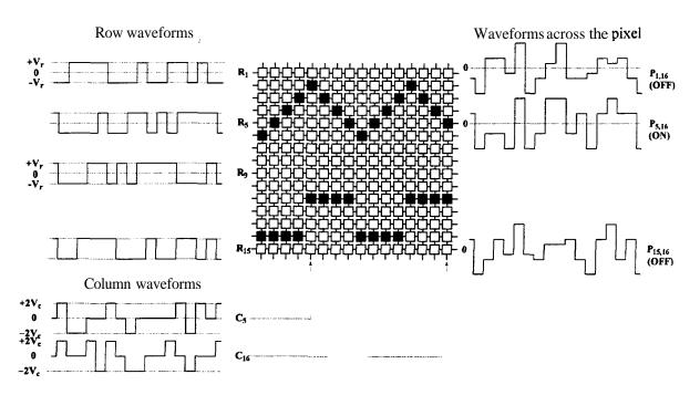
Figure 2-41 Typical addressing waveforms of PRBS-PC.
