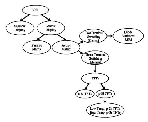
Figure 2-3 Different types of liquid crystal displays.
