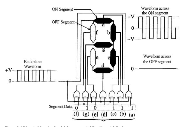
Figure 2-1 Direct addressing for driving segmented liquid crystal displays.
