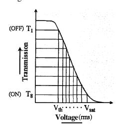
Figure 2-24 Schematic representation of electro-optic characteristics of liquid crystal display.
