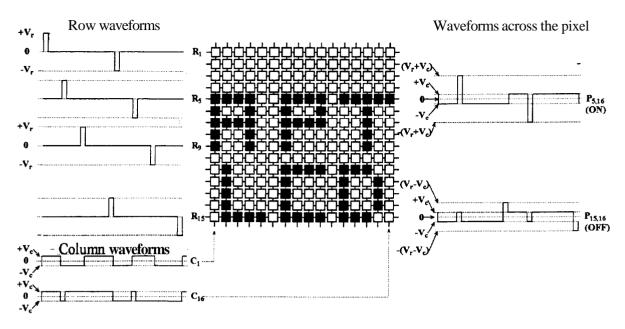
Figure 2-5 Typical addressing waveforms of APT
