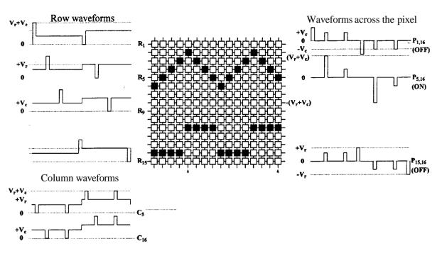
Figure 2-39 Typical addressing waveforms of modified RPAT-PC.
