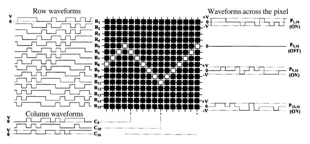
Figure 2-34 Typical addressing waveforms for displaying single waveforms selecting all the rows using pseudo random sequence.
