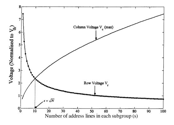
Figure 2-21 Row voltage  $(V_c(max))$  for N = 100 versus number of address lines selected simultaneously (s).
