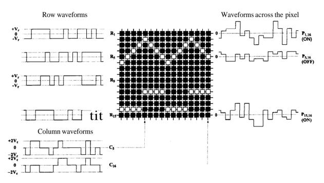
Figure 2-40 Typical addressing waveforms of PRBS-NC.
