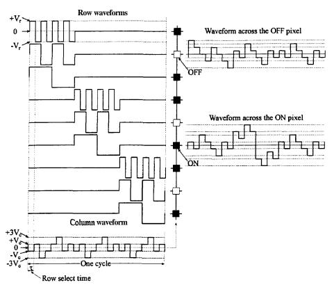
Figure 2-12 Typical addressing waveforms of IHAT, for *N*=9 and *s*=3.
