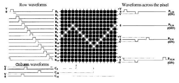
Figure 2-33 Typical addressing waveforms to display single waveform
