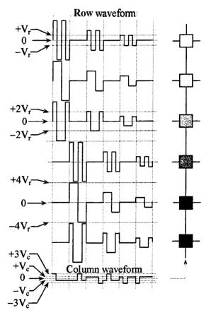
Figure 2-32 Typical addressing waveforms of row pulse height modulation using multi-line addressing technique.
