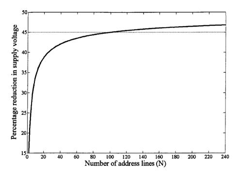
Figure 2-9 Percentage reduction in supply voltage of IAPT as compared to APT for various values of  $N_{\bullet}$
