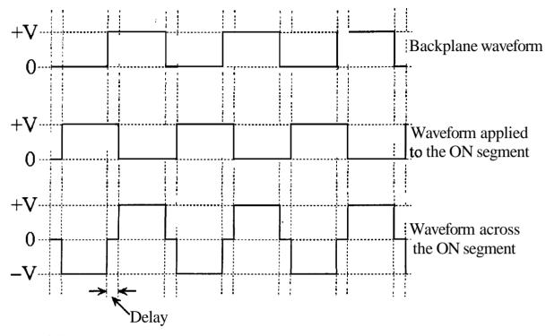
Figure 2-2 Addressing waveforms used to reduce the power consumption in direct addressing.
