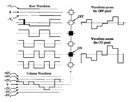
Figure 2-23 Typical addressing waveforms of active addressing technique.
