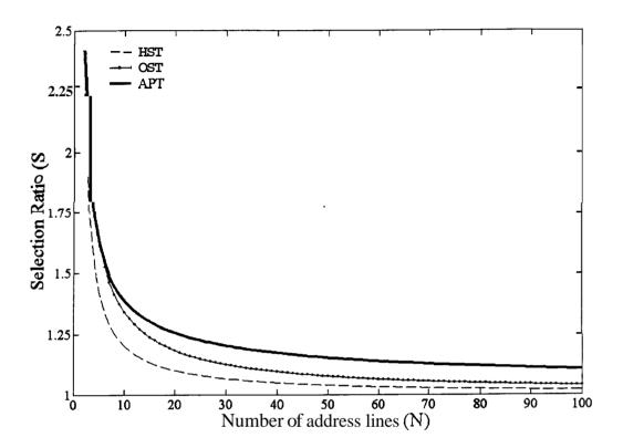
Figure 2-6 Selection ratio versus number of address lines for Half select, One-third select and Alt and Pleshko addressing techniques
