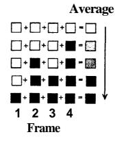
Figure 2-27 Generating gray shades using frame rate control.
