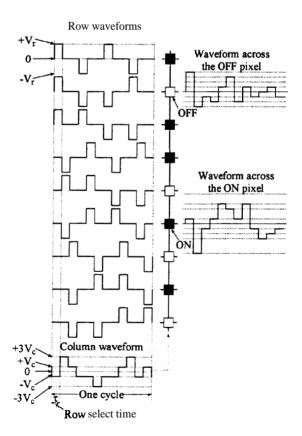
Figure 2-20 Typical addressing waveforms of MLA while selecting three rows at a time.
