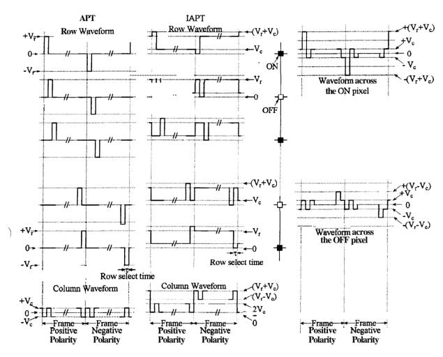
Figure 2-7 Typical addressing waveforms of APT and IAPT.
