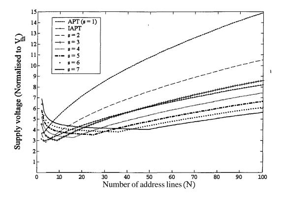
Figure 2-22 Supply voltage (normalized to  $V_{th}$ ) versus N for various values of s.
