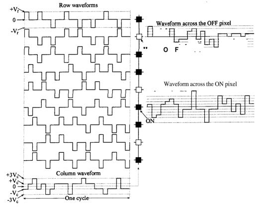
Figure 2-14 Typical addressing waveforms of IHAT (N = 9 and s = 3), row select pulses are changed whenever a new subgroup is selected.
