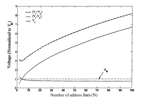
Figure 2-11 Instantaneous voltage across the ON and OFF pixels (normalized to  $V_{th}$ ) versus number of address lines (N).
