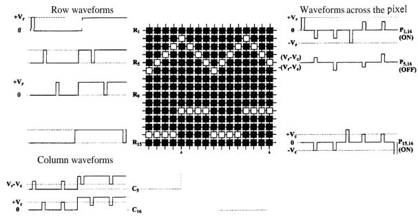
Figure 2-38 Typical addressing waveforms of modified RPAT-NC.
