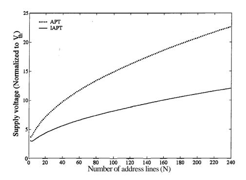
Figure 2-8 Supply voltage (normalized to  $V_{th}$ ) versus number of address lines of APT and IAPT
