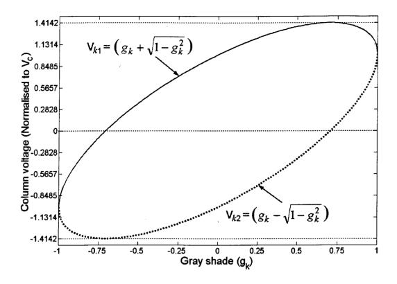
Figure 2-29 Column voltage (Normalized to  $V_c$ )  $V_{kl}$  and  $V_{k2}$  in to time intervals t1 an t2 for displaying gray shades using split interval amplitude modulation technique.
