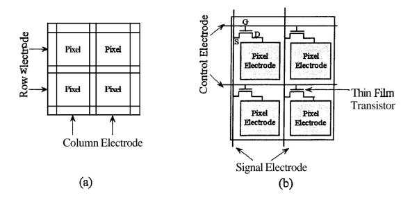
Figure 2-4 Schematic representation of (a) passive matrix (b) active matrix liquid crystal displays.
