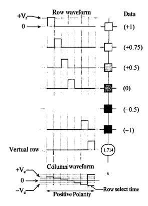
Figure 2-30 Typical addressing waveforms of full interval amplitude modulation technique for displaying gray shades by selecting one row at a time.
