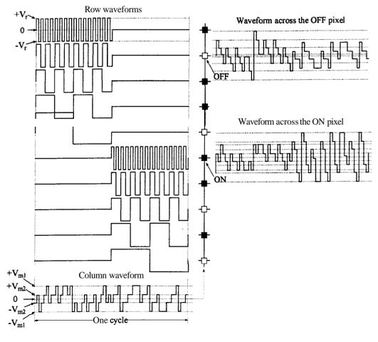
Figure 2-17 Typical addressing waveforms of IHAT-S4, for N=10 and s=5.
