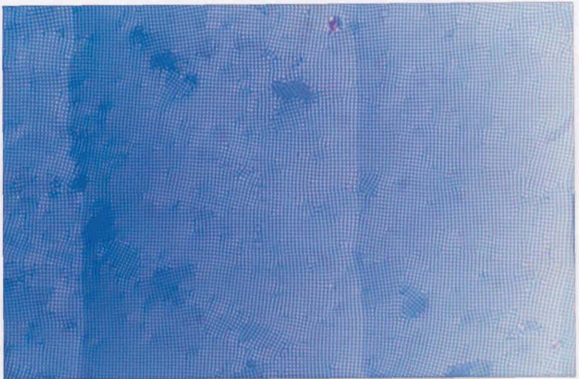
Figure 4.13: (a) Photograph of the TGB_A texture in a wedge shaped cell. The vertical lines are the GC lines, which indicate that there is a twist deformation in the director along the normal to the glass plates, ie. along the viewing direction. (b) The same region, recorded after the transition to the square grid texture was complete. The grid spacing is about 2\mu m . The GC lines are clearly visible. The increase in the spacing between the GC lines compared to the TGB_A case shows that the pitch of the structure is larger than that of the TGB_A . The colour variation is also due to this reason.
