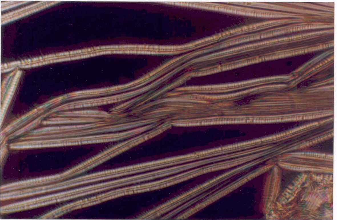
Figure 4.26: (a) The TGB_A filaments in the absence of any external field and (b) after the same region was cooled to the new phase and a field of \sim 5V/\mu m was applied between the ITO coated plates.
