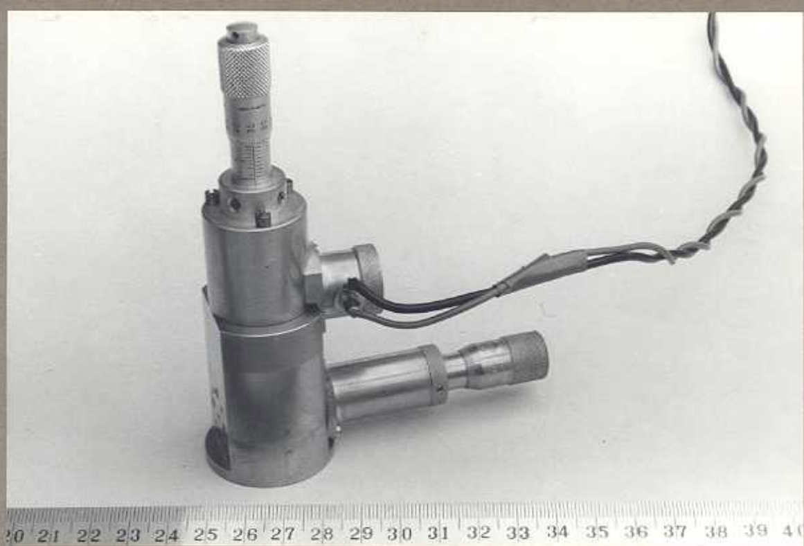
Figure 2.6 (a): A fully assembled Gunn oscillator.
