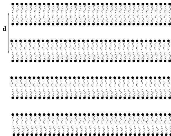
Figure 1.9: Schematic diagram of the lamellar phase which consists of bilayers stacked one above the other. d is the lamellar periodicity.
