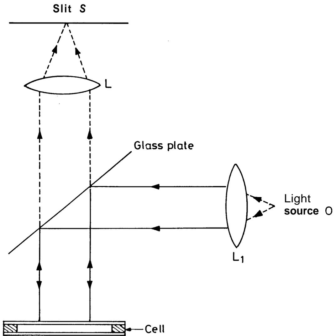
**Figure 2.12.** Arrangement to measure the thickness of the cell by forming the channelled spectrum.
