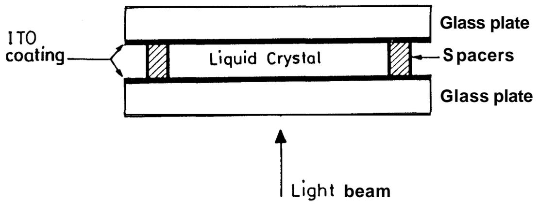
**Figure 2.11.** Geometrical configuration of the cell.
