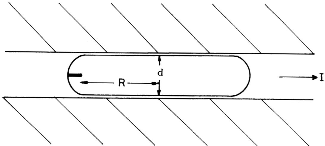
**Figure 2.2.** Vertical cross-section of a flattened cholesteric droplet between two glass plates. It is surrounded on all sides by the isotropic phase.
