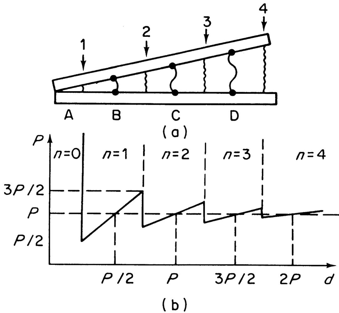
**Figure 2.7.** (a) Wedge shaped cell. The numbers indicate Cano-Grandjean disclinations and the letters indicate the Grandjean zones. (b) Calculated dependence of the forced pitch upon the thickness of the cell.  $n$  is the number of half-turns of the helix in a Grandjean zone. (From Blinov, 1983).
