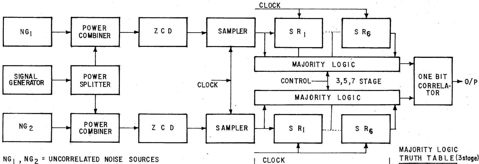
FIG. A . 4 AN EXPERIMENTAL SET UP TO DEMONSTRATE THE FILTERING ACTION OF ONE BIT FILTERS
