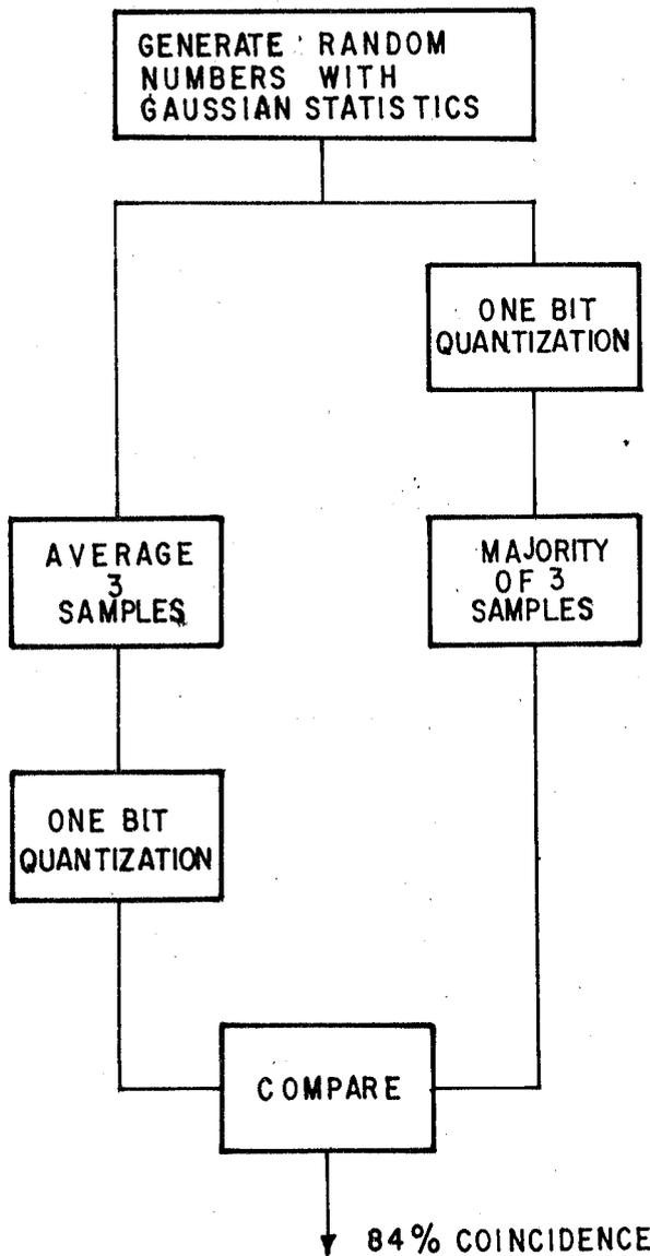
FIG. A . 6 SCHEME TO STUDY THE SIMILARITY BETWEEN MULTIBIT AND ONEBIT, 3 STAGE FILTERS
