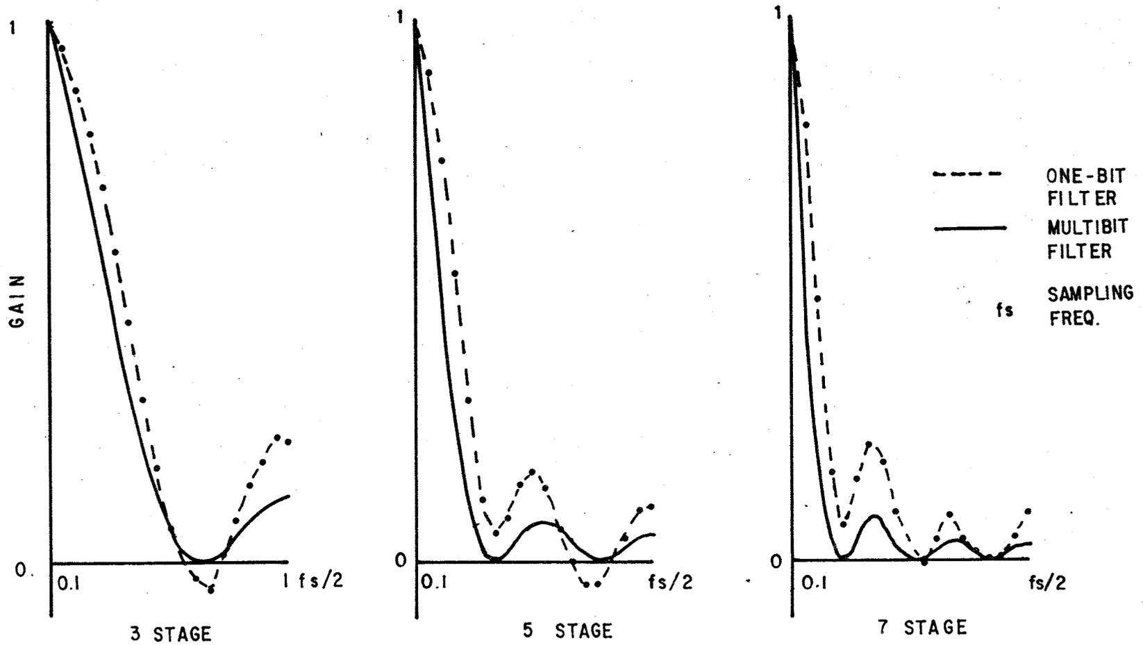
FIG.A.5 FREQUENCY RESPONSE OF MULTIBIT & ONE-BIT DIGITAL FILTERS
