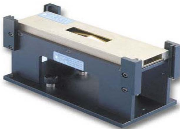
*Figure 11: FT-85 accessory used for the grazing angle FTIR spectroscopy*
