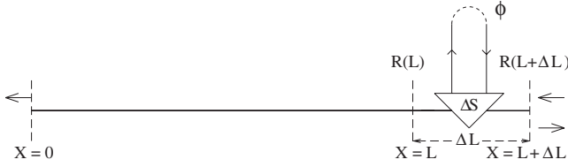
FIG. 2. A schematic description of the “invariant embedding” method for a 1D conductor with random-phase reservoirs distributed uniformly along the length.
