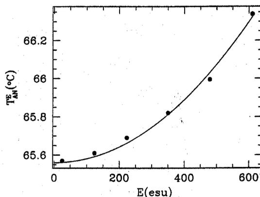
Figure 5:  $T_{AN}^E$  as a function of applied electric field in 8OCB. The symbols are experimental data. The calculated variation corresponds to the prediction of the Landau theory that the shift in transition temperature is proportional to  $E^2$ .
