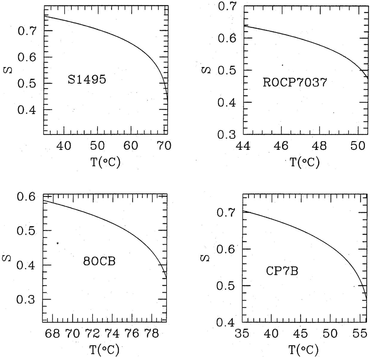
Figure 11: Order parameter measured using the magnetic susceptibility data as a function of temperature.
