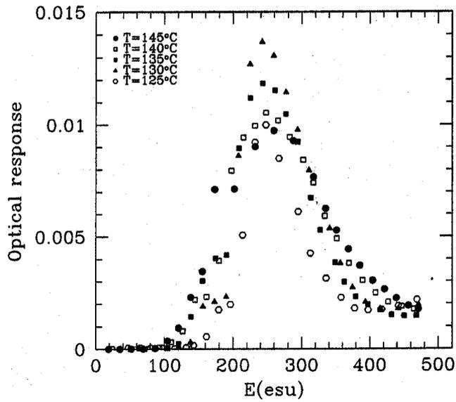
Figure 9: Optical response of pentyl cyanoterphenyl (5CT) as a function of field at different temperatures.
