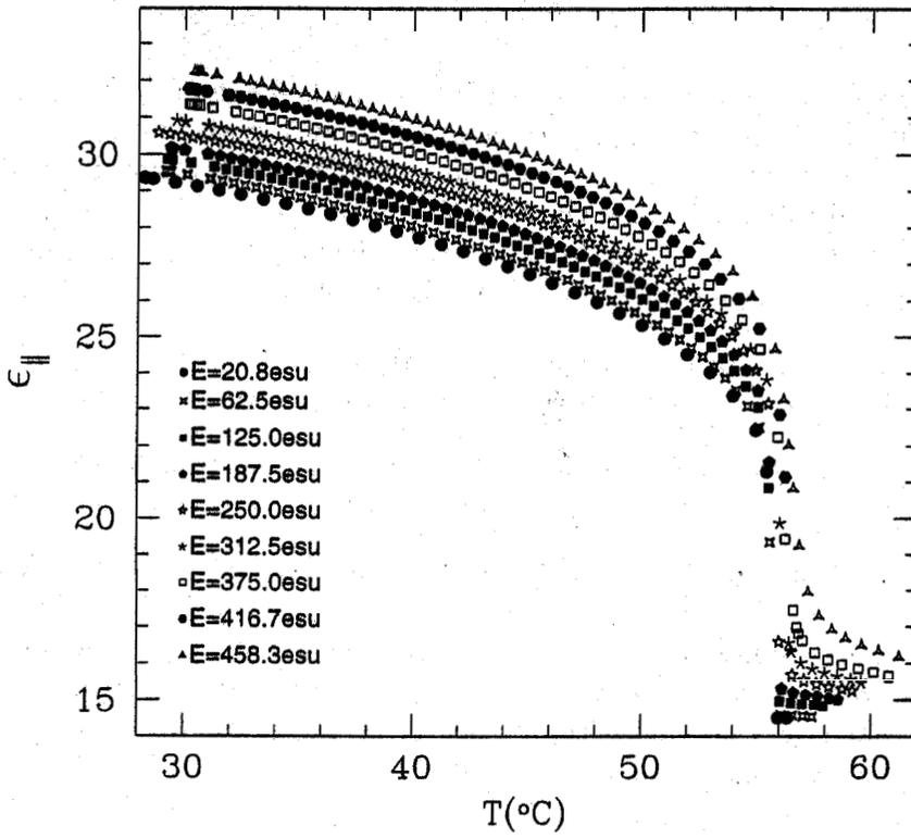
Figure 7: Variation of  $\epsilon_{\parallel}$  as a function of temperature in nematic range of CP7B at different fields  $d=16 \mu\text{m}$ ,  $f=4111\text{Hz}$
