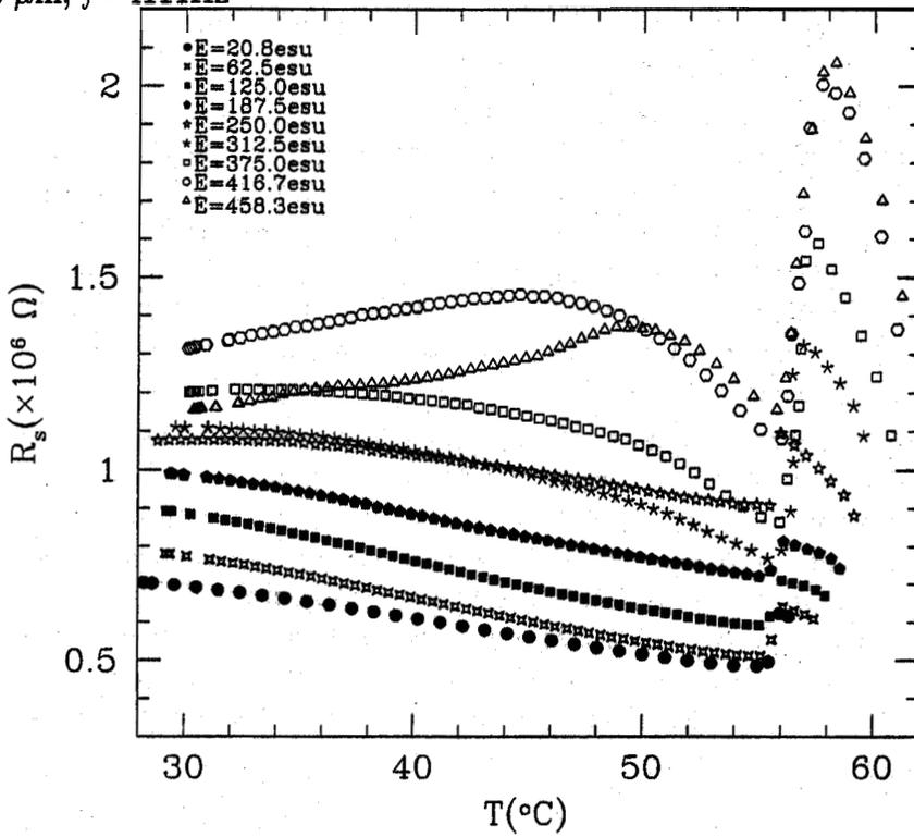
Figure 8: Temperature variations of the resistance of a  $16 \mu\text{m}$  thick sample of CP7B at various values of the applied electric fields.
