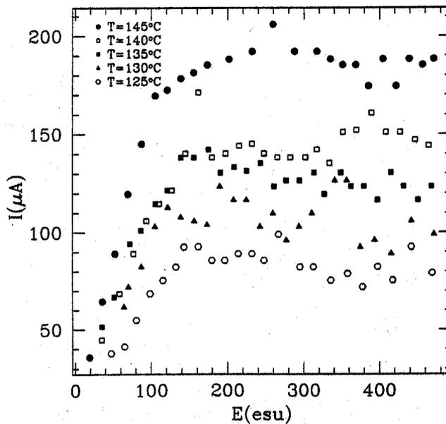
Figure 10: Current measured in a 5CT sample cell as a function of field at different temperatures.
