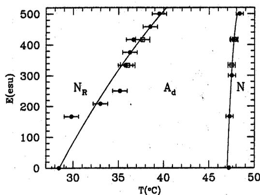
Figure 6: The electric field phase diagram for the 60CB - 80CB mixture. Circles are data obtained from light scattering measurements and open squares are those obtained from the electrical impedance measurements. The solid lines are guides to the eye. Note that the data on the  $N_R$ - $A_d$  transition are consistent with a change of slope around 200 esu.
