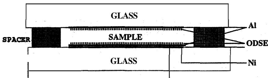
Figure 2: A side view of the constructed cell.
