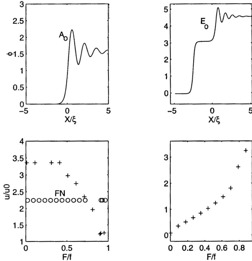
Figure 4.3: Solitons with a tapered lattice. (a) The  $A_0$  type of soliton (b)  $E_0$  type of soliton. Scaled velocity  $u$  of a soliton as a function of scaled force for (c)  $A_0$  soliton and (d) for  $E_0$  soliton.
