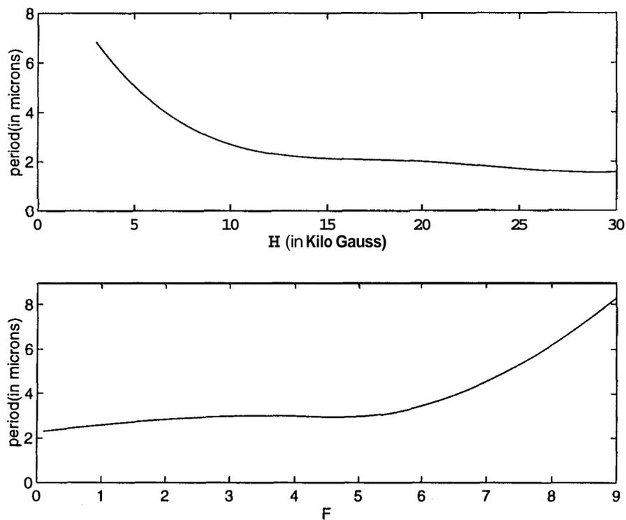
Figure 4.5: *Period dependance of the tapered lattice on(a)  $F$  and (b) on  $H$ . For  $H < H_c$  we have asynchronous regime*
