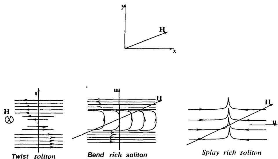
Figure 4.2: *Dynamic single solitons in a ferronematic in a rotating field ( $H$ )*
