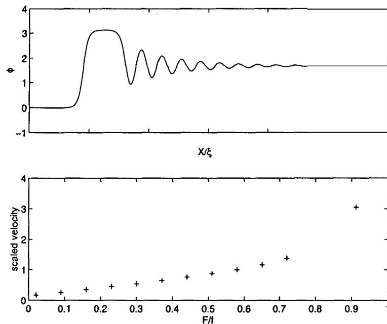
Figure 4.4: A  $G_0$  soliton with its velocity-force characteristics.
