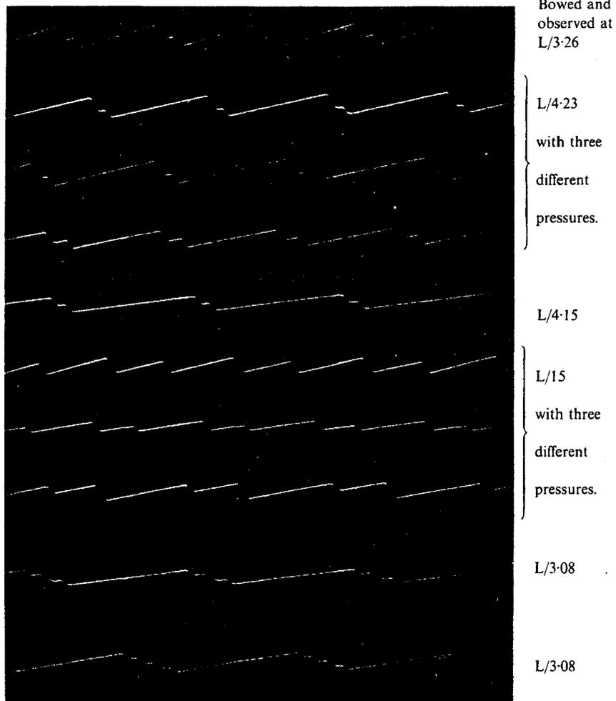
**Plate IX.** Modified four-, six-, and eight-step zig-zag vibration-curves at the bowed point, showing the practical constancy of the velocity of ascent with the bow, and the variability of the velocity of descent against the bow.
