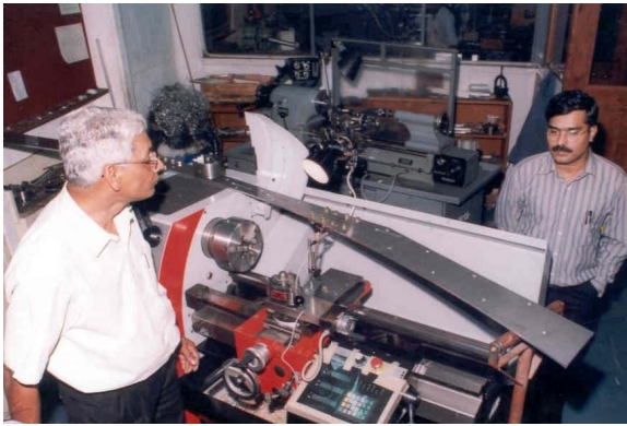
Fig. 7. A photo showing the profile segments, ground keys, slots and side-plates to ensure alignment.
