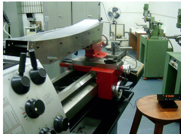
Fig. 10. A photo showing mirror, formed by cladding a 1 mm thick sheet over the substrate made by assembling the two end laminates in parallel and aligned using ten spacers, on the test bed.
