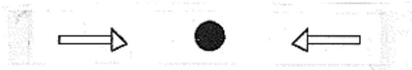
Figure 2. a , A cloud of ^{87}\text{Rb} atoms placed between two counter-propagating red detuned laser beams.
